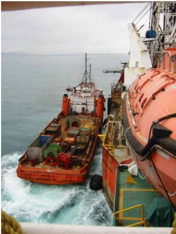
Figure 20, Relative DP operation between two moving vessels.
