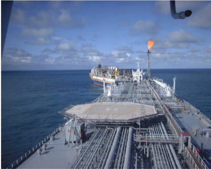
Figure 19, Offloading tanker connected to Norne
