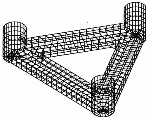
**Figure 8. The triangular semi-submersible : discretization**
