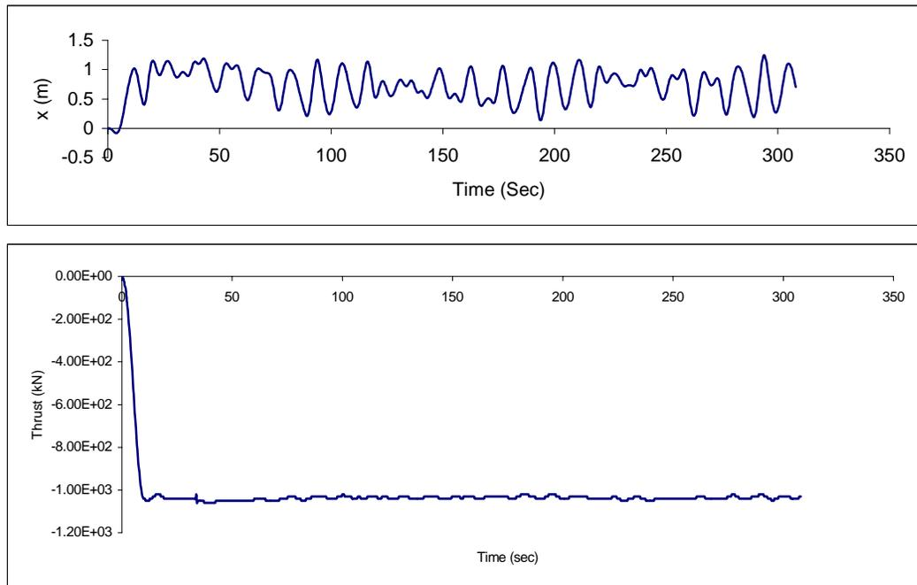
**Figure 5. Surge displacement and DP thrust;  $H_s = 4\text{m}$ , heading =  $0\text{deg.}$ , current =  $1\text{m/s}$ , initial steady mean thrust of 1000 kN.**
