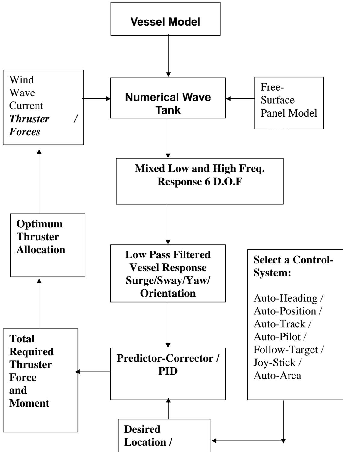
Figure 1 Numerical Wave Tank Simulation of DP System
