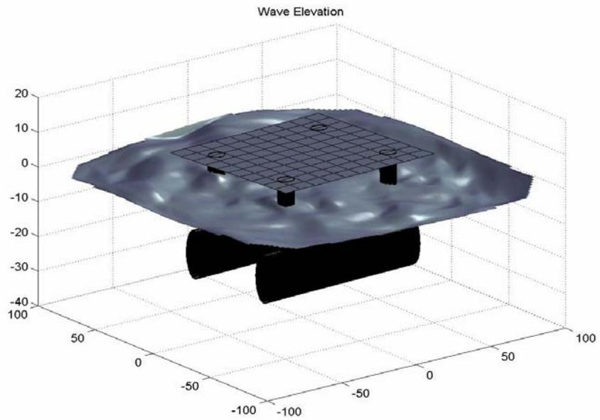
**Figure 2. A 3D View of the Semi-submersible in Numerical Wave Tank Simulation for Random Waves**
