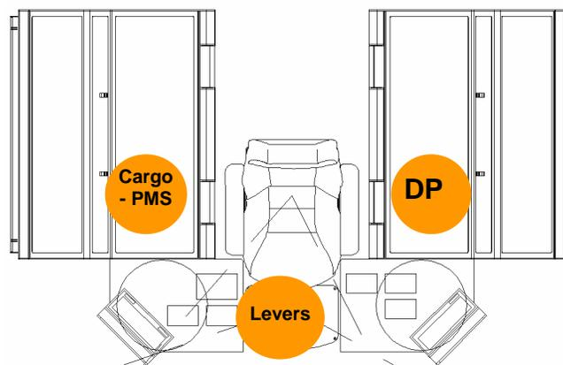
Figure 9 - Basic layout of the specialized operator position
