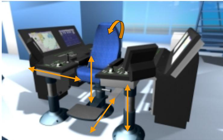
*Figure 10 – An adjustable workplace*
