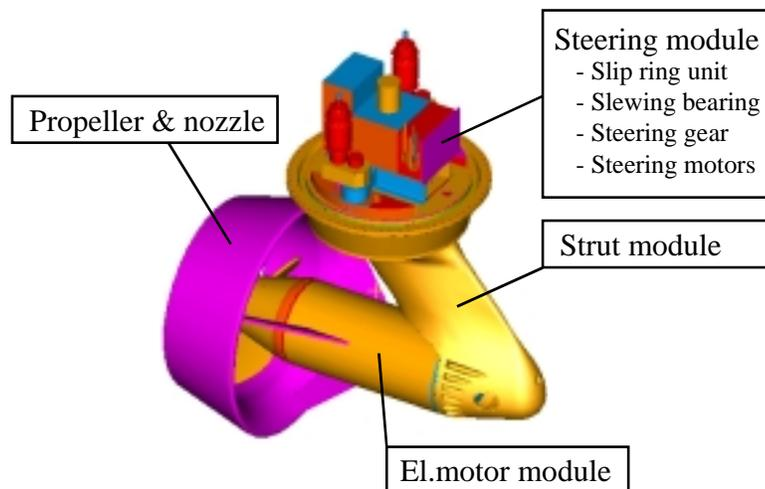
Fig. 4: Compact Azipod thruster.
