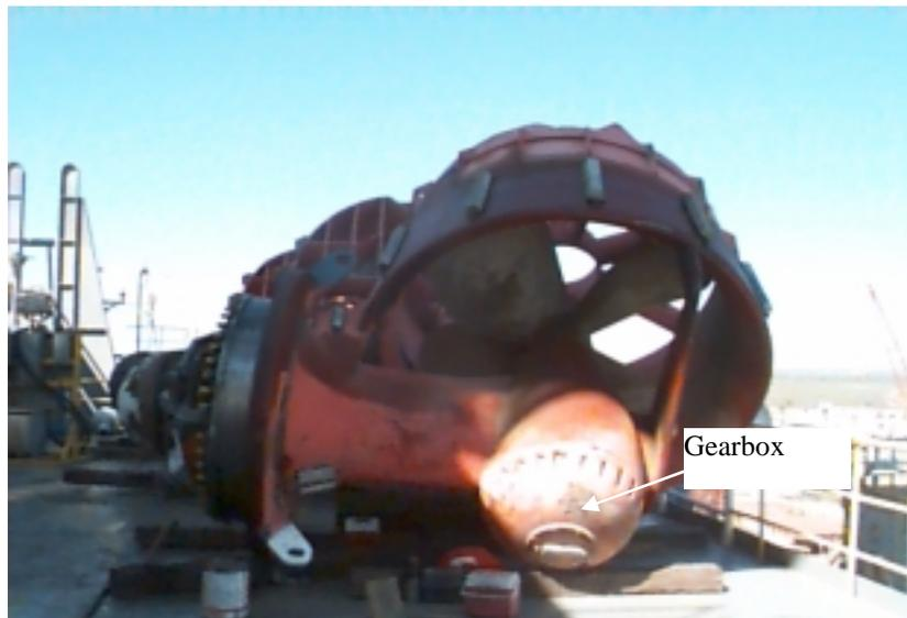
Fig 2: Typical azimuthing thruster
