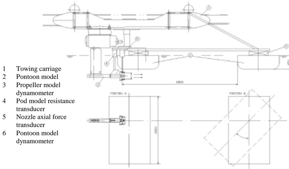
Fig. 13: Experimental setup for determination of interaction between thruster and platform hulls.
