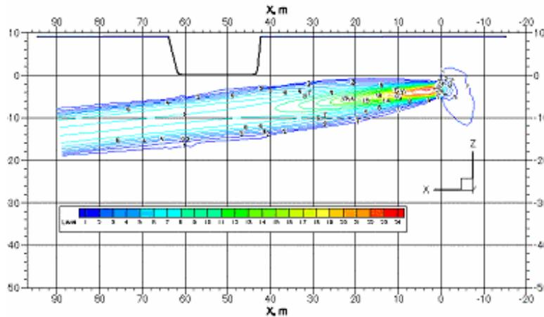
Fig.12. Impact of the propeller jet to pontoon B, showing the axial velocity  $V_x$  distribution through the center of the propeller disk.
