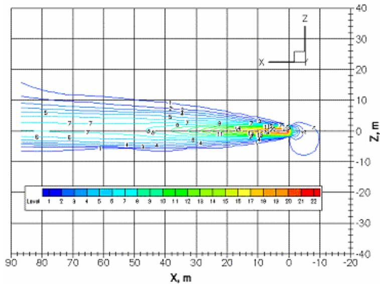
Fig. 9: Distribution of axial velocity  $V_x$  in propeller jet. Full scale condition.
