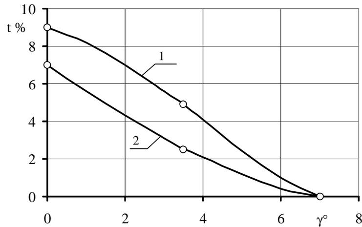
Fig. 16: Thrust deduction coefficient as a function of the tilt angle when the jet is directed along the hull.
