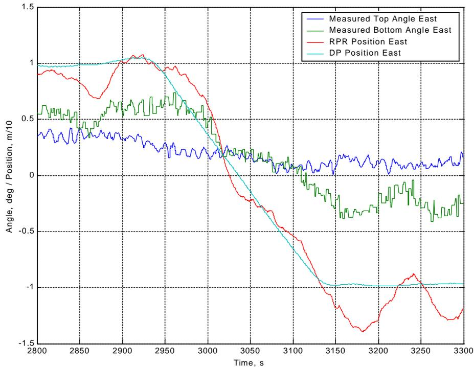
It is interesting to note that the upper flex joint inclination is quite insensitive to the move, compared to the lower flex joint. This is because a deepwater drilling riser behaves more like a catenary (chain) rather than a rigid beam.
