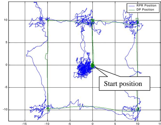
Later the RPR was used together with DGPS and LBL to see whether the DP accepted it as a valid reference or not. This test turned out successfully. We observe, however, that the RPR is affected by significant colored noise caused by the riser dynamics, which cannot be fully filtered out.
