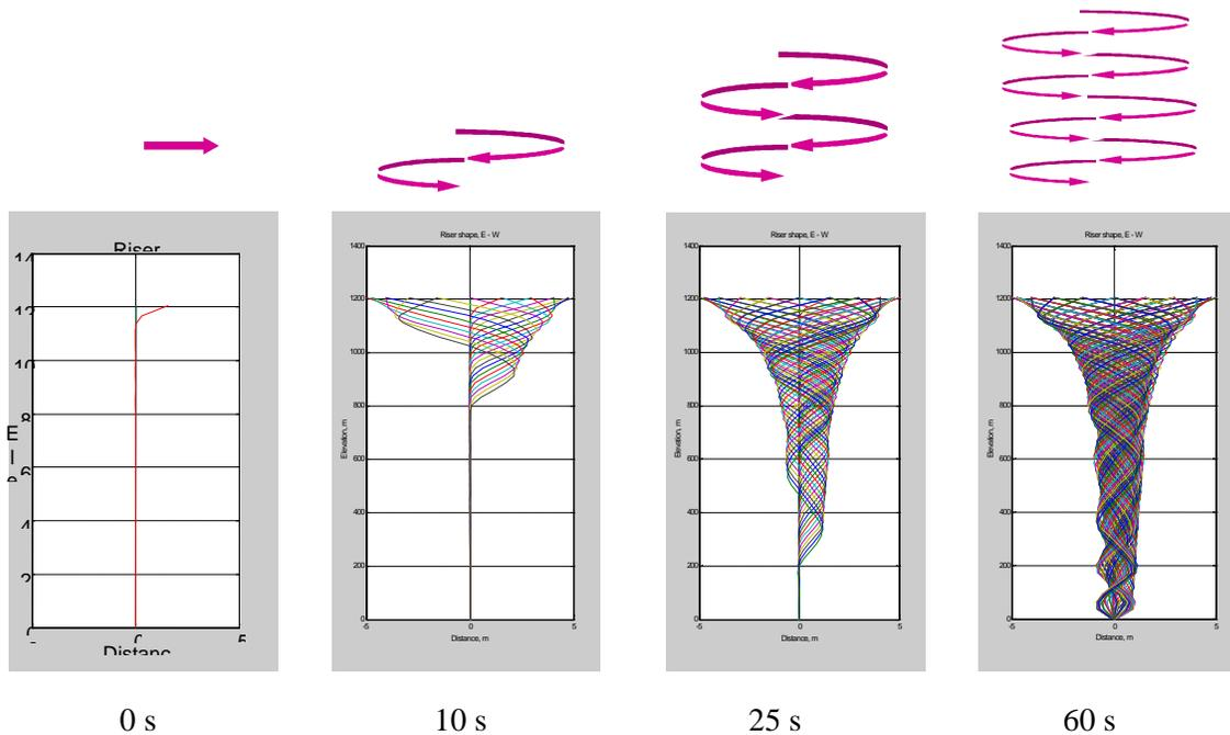
The inclination measured of the lowermost riser joint (just above lower flex-joint) will reflect the most slowly varying components of the horizontal motions of the vessel (including steady position offset) and the actual current profile. Most of the 1<sup>st</sup> order vessel motions will be filtered out mechanically at this location.
