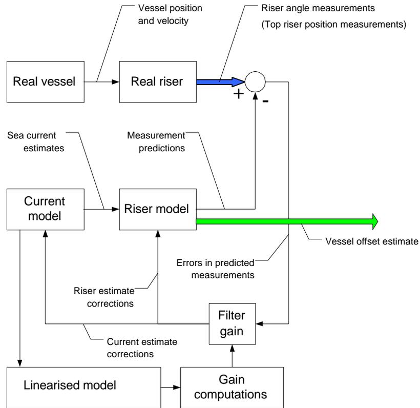
The blue arrow represents the riser input: upper and lower riser inclinations. The green arrow indicates the output: the real-time estimate of vessel position relative to the well head.
