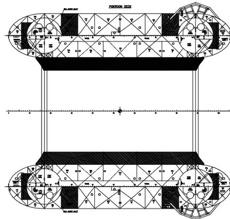
**Figure 3** Lower hull extensions and new thruster rooms
