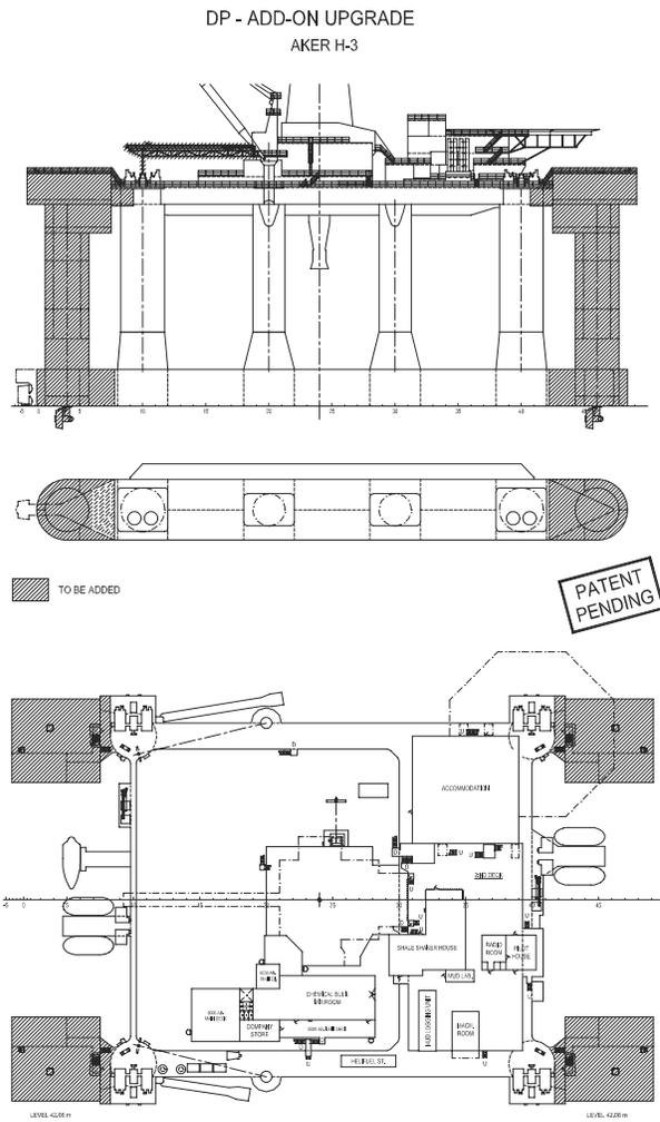
Figure 6 "DP-Add-On" Upgrade for an Aker H3
