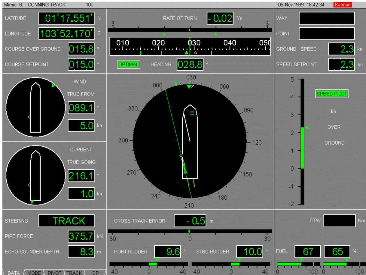
All advanced functionality is present through the VDU display. This provides automatically all information that is relevant for the selected operation mode. In addition, it provides access to the advanced functionality of the DpDt system.
