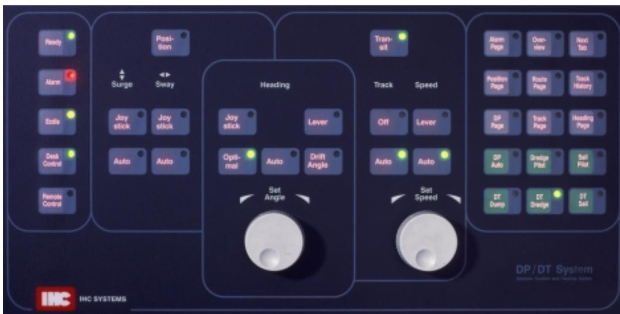
A new command panel has been designed with a minimum amount of buttons and signal lamps. The functionality is limited to the bare essentials, not much more than auto / manual selections of the available control modes and some status indications. In addition, the DpDt system uses the available manual control components (steering wheel, levers) as inputs.
