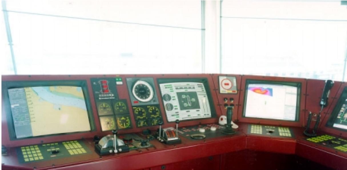
It is designed to have a centralized position within the navigation console. That way, switching over between manual and automatic control can be performed without changing control position. By placing the DpDt system in such a centralized position the controls for manual operations (steering wheel, levers for propulsion and bow winches) can also be used in semi-automatic modes.
