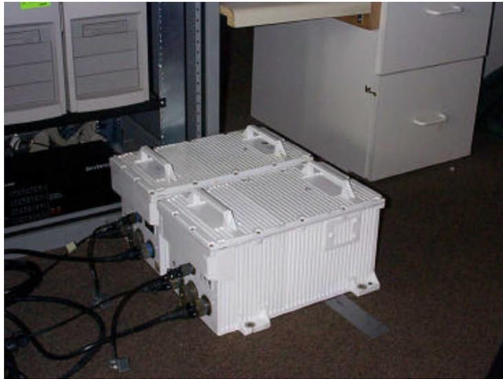
Fig. 13 Dual IMU set up for offshore testing
