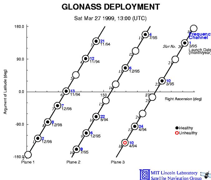
**Figure 2.** GLONASS constellation showing the recent launch of three vehicles (2, 7, and 8) into Plane 1 (MIT Lincoln Lab).
