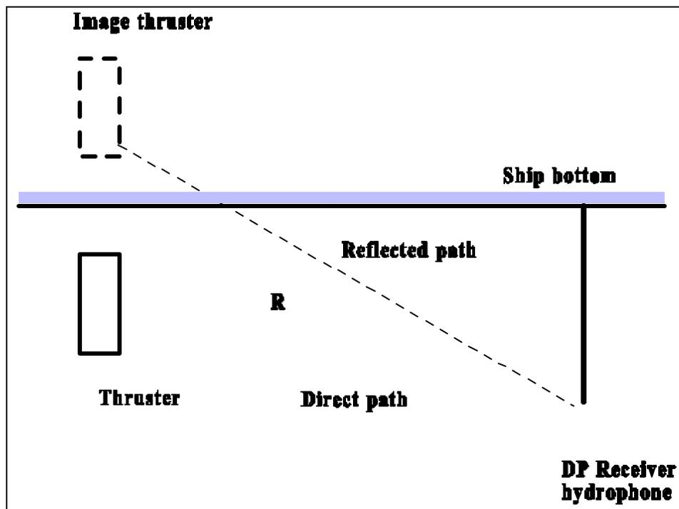
estimated. Note that, because of efficient reflection from the ship's bottom at shallow grazing angles, there are two paths for noise transmission for each thruster-hydrophone pair; see figure 2. Effectively, the number of thruster sources is doubled, but the reflected path has a transmission path approaching the hydrophone at a higher elevation angle.
