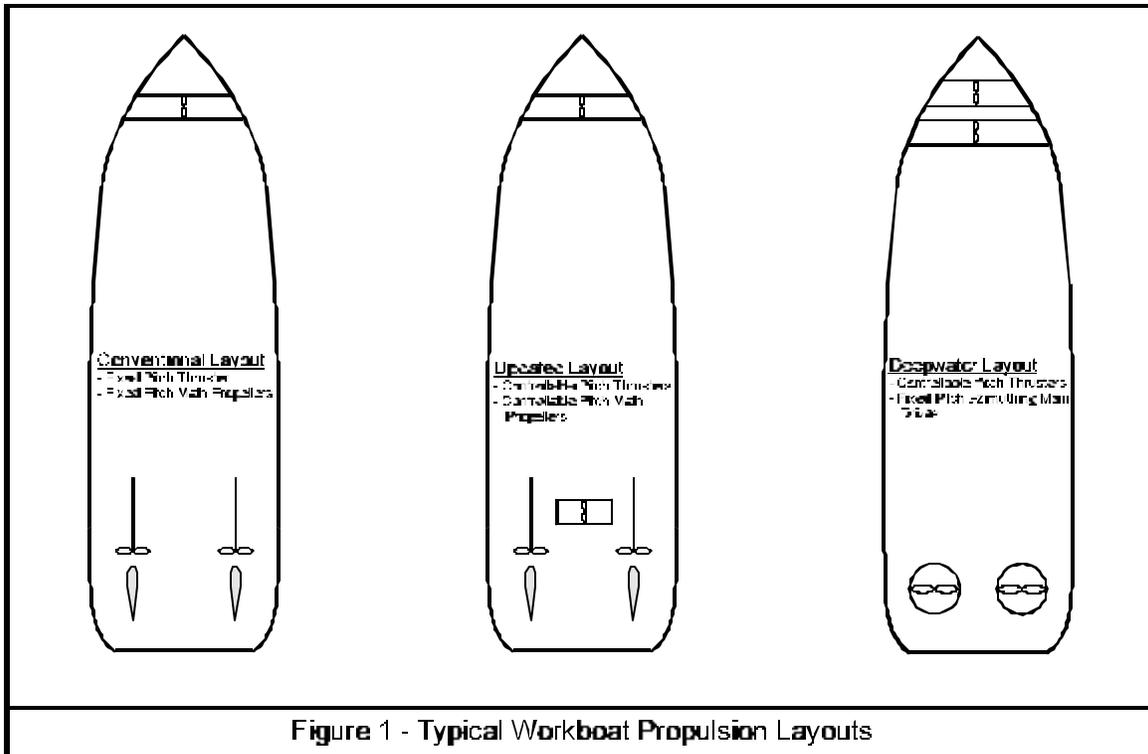
**Figure 1 - Typical Workboat Propulsion Layouts**
