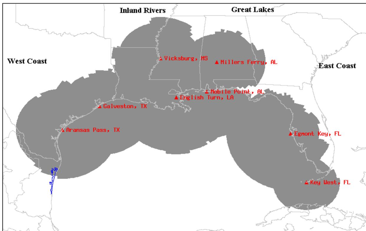
**Figure 1 - USCG DGPS Service Coverage Area**
