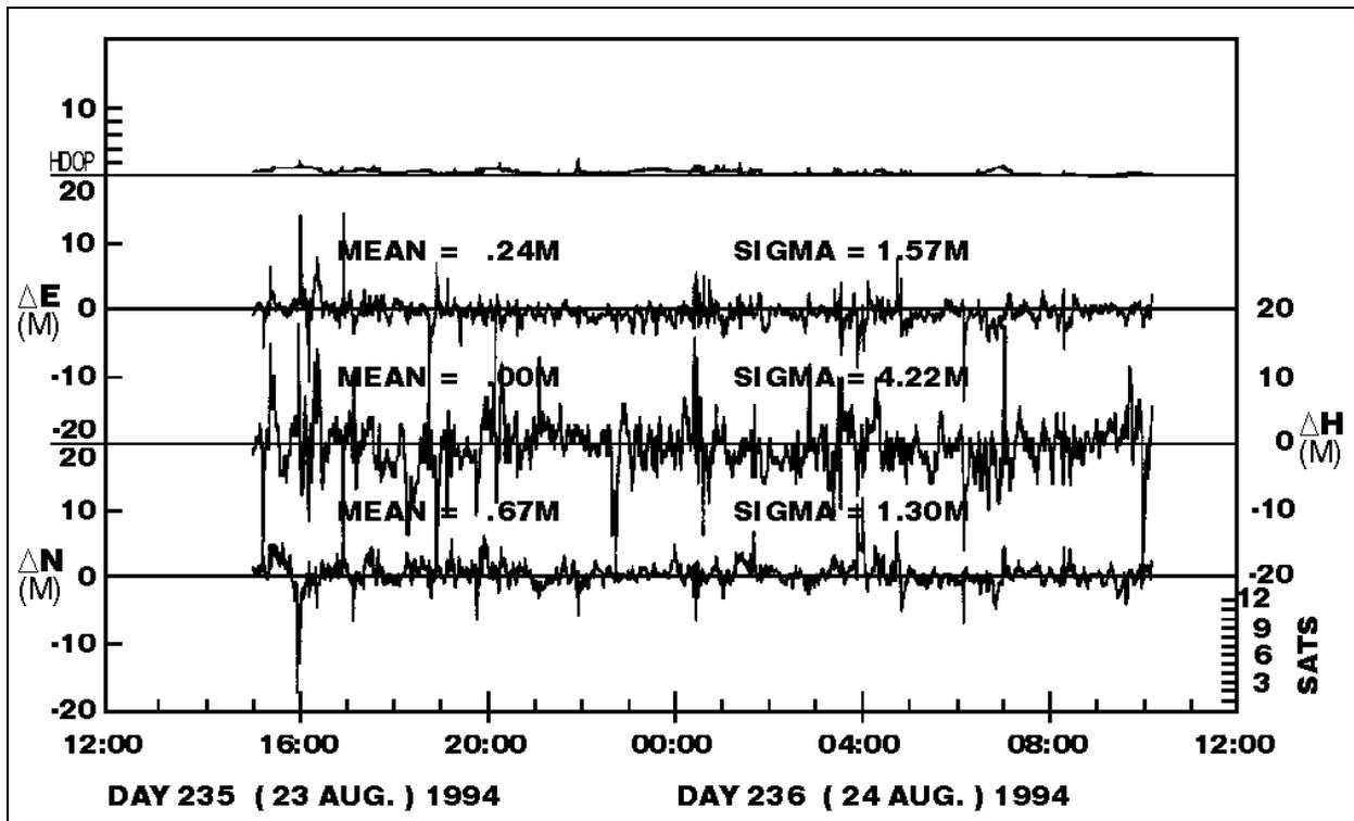
Figure 4 - DGPS Position v. Time
