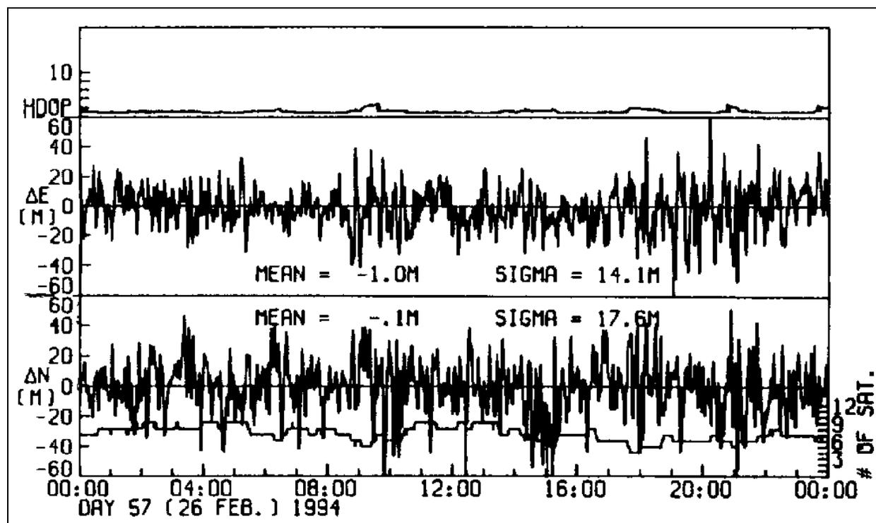
Figure 3 - Uncorrected GPS Position v. Time
