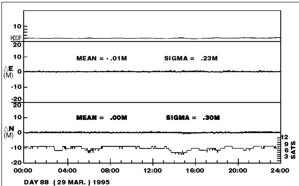
Figure 5 - Survey-quality DGPS Position v. Time
