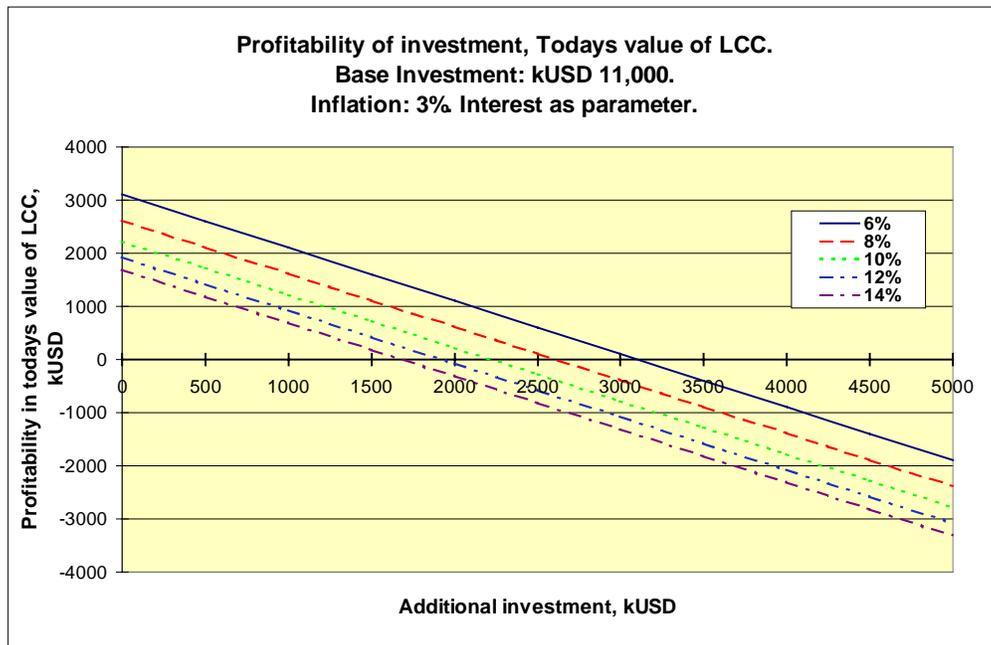
Fig. 10: Investment analysis (Life Cycle Cost - LCC) for variable-speed FPP thrusters vs. constant-speed CPP thrusters for a floating production vessel. The curves show the profitability of the difference in investment between a constant-speed and a variable-speed thruster drive configuration. For this special application, the difference in investment cost is kUSD 2-2.5, hence at break-even with an interest rate of 10%.
