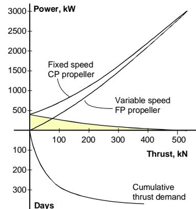
(b): Typical CPP and FPP characteristics and cumulative thrust demand.
