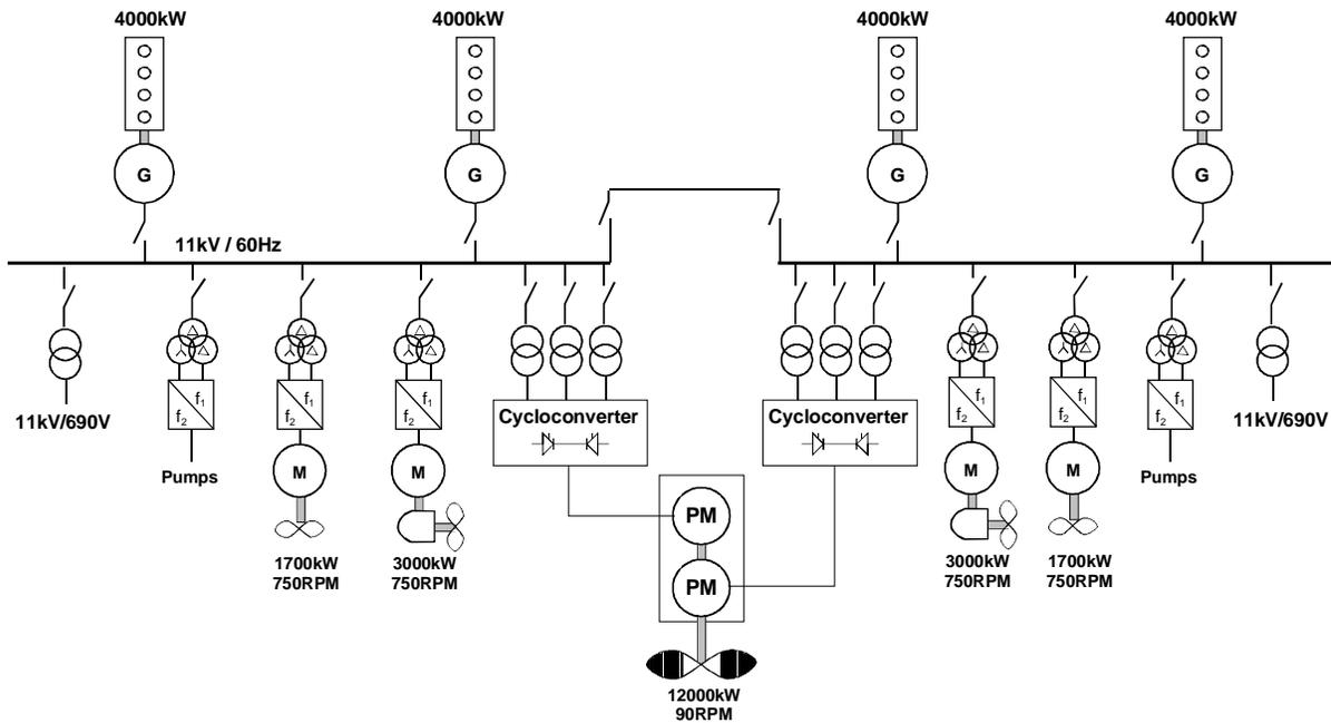
Fig. 3. Shuttle tankers: A typical power system configuration for a DP shuttle tanker.
