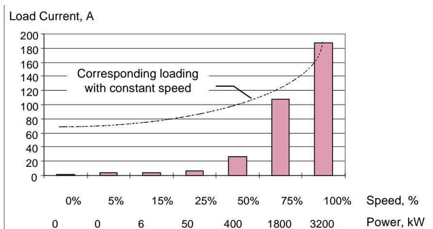
Fig. 11: Drive load current for a 3200 kW PWM variable-speed drive (VSD) compared with a constant-speed CPP thruster.
