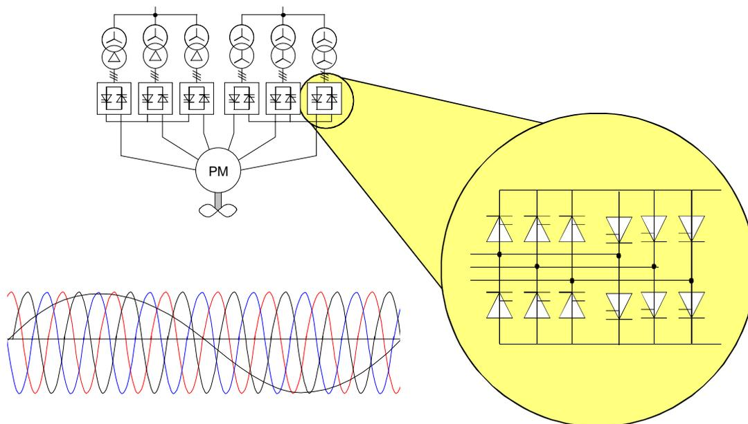
*Fig. 7: Cycloconverter drive with input and fundamental output waveforms. The output voltage is constructed by selecting phase segments of the supply voltage.*
