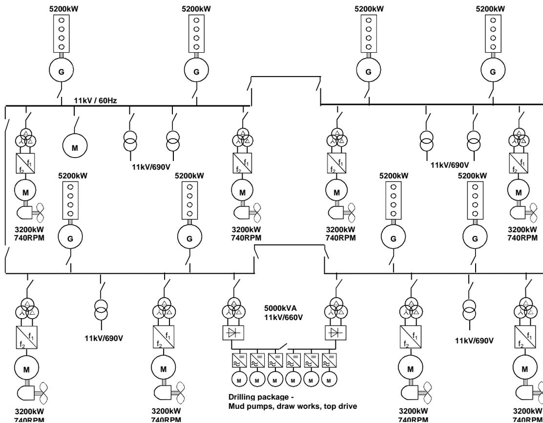
Fig. 1. Drilling vessels: A typical power system configuration for a DP Class 3 drill rig with a four-split power system.
