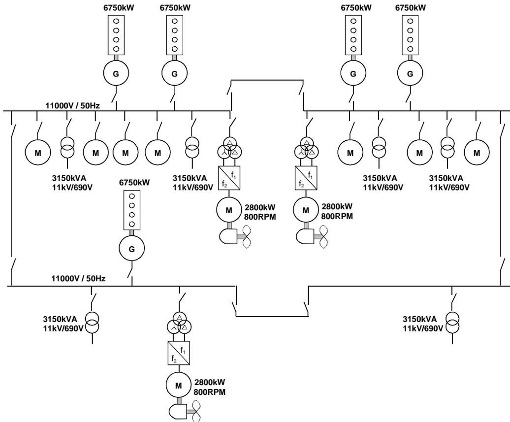
Fig. 2. Floating production: A typical power system configuration for thruster-assisted position-moored FPSOs with a two-split main switchboard configuration and emergency switchboard.
