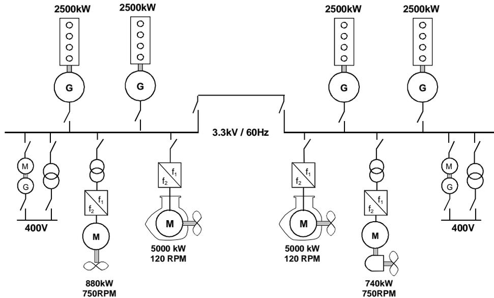
Fig. 4: Service vessels: A power system configuration for a supply vessel.
