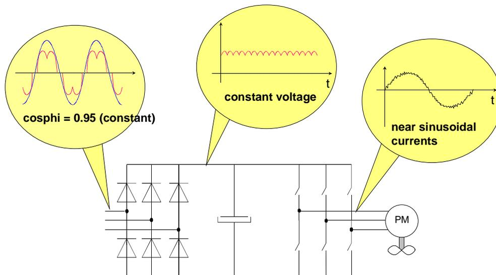
Fig. 8: Two-level PWM drive.
