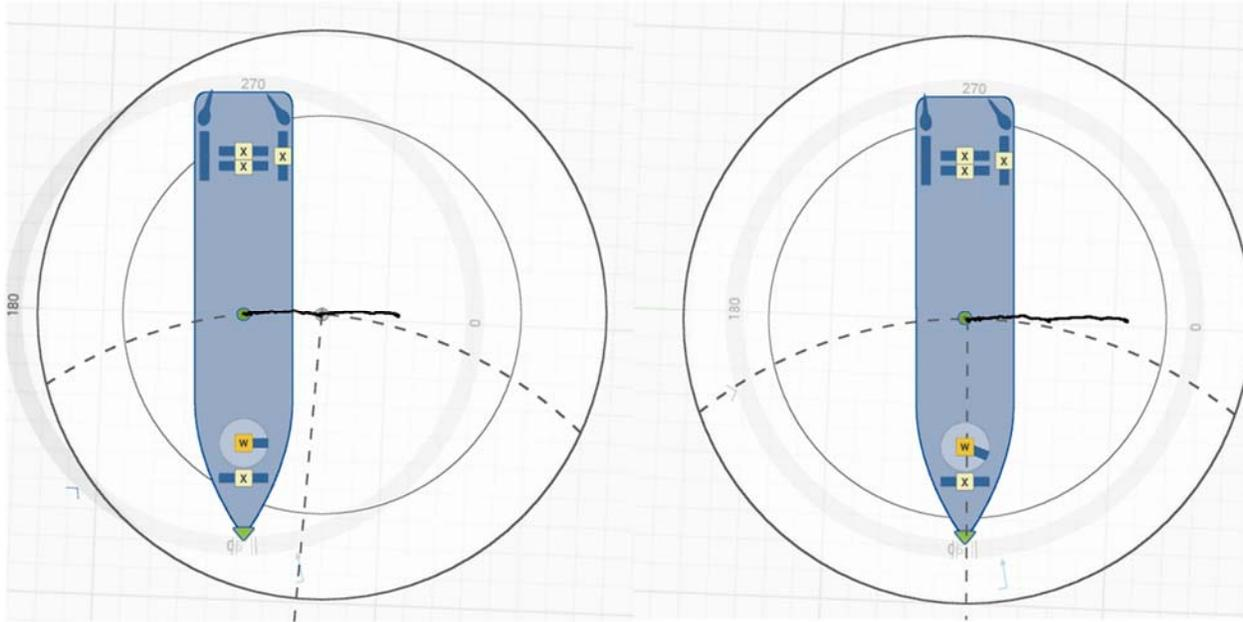
Weather-optimal positioning finds the vessel heading and position that requires the least amount of energy to stay on spot and provides a great potential for improved fuel efficiency. However, it will be more energy-efficient when combined with other measures. With WOP, the vessel is able to keep the position in the watch circle with a limited thruster configuration. The reduced demand for energy lets the operator use thrusters such that the minimum amount of power generators need to be running.
