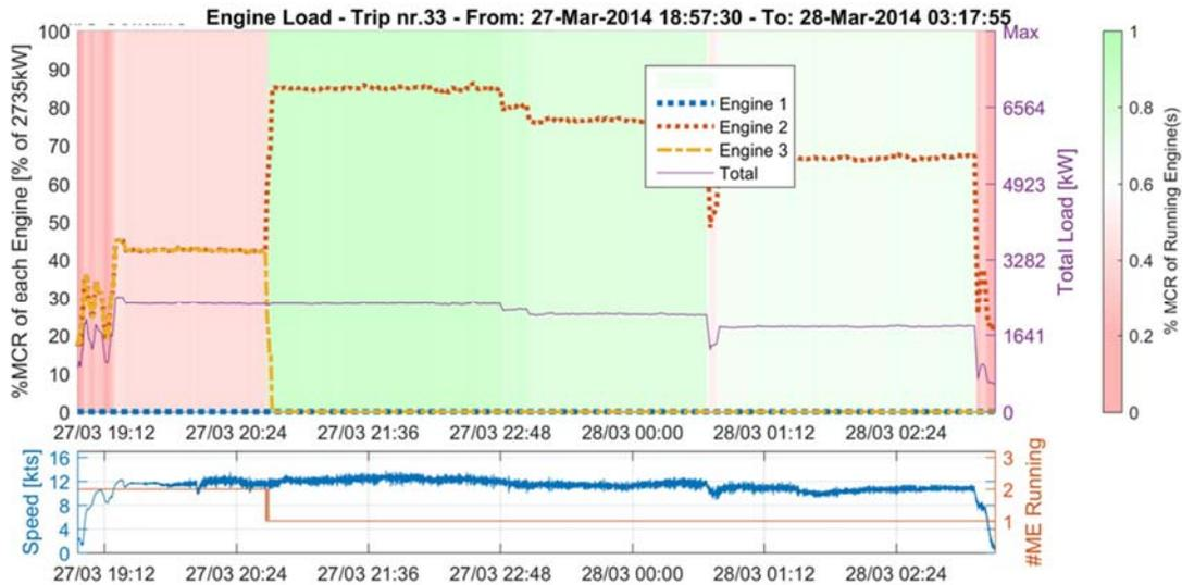
Another ship-owner used the logged data to negotiate a contract with new operational terms with a charterer. The old terms required all engines to be running during operations. The analysis showed the average and maximum load on each engine during normal operational procedures and convinced the charterer to reduce the amount of running engines. The change improved engine load and decreased fuel consumption
