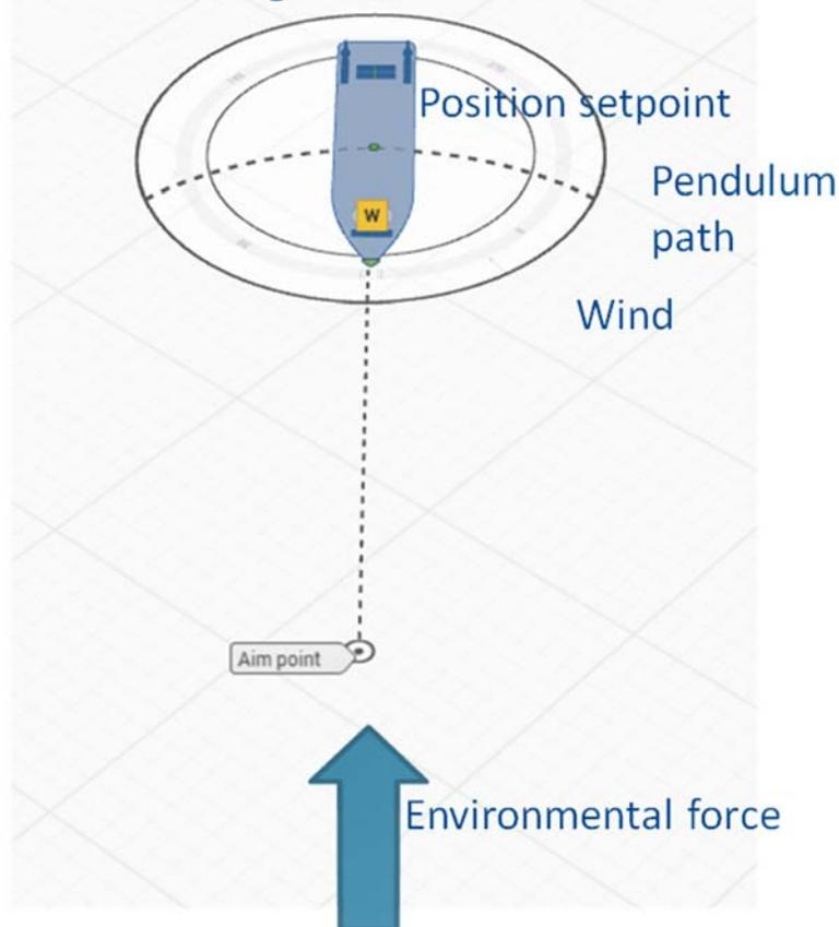
The system maintains a heading and position precision within a prescribed area during operation but there are limitations on absolute position certainty. Given safety restrictions, we see that such a system is most suitable for standby operations for longer periods.
