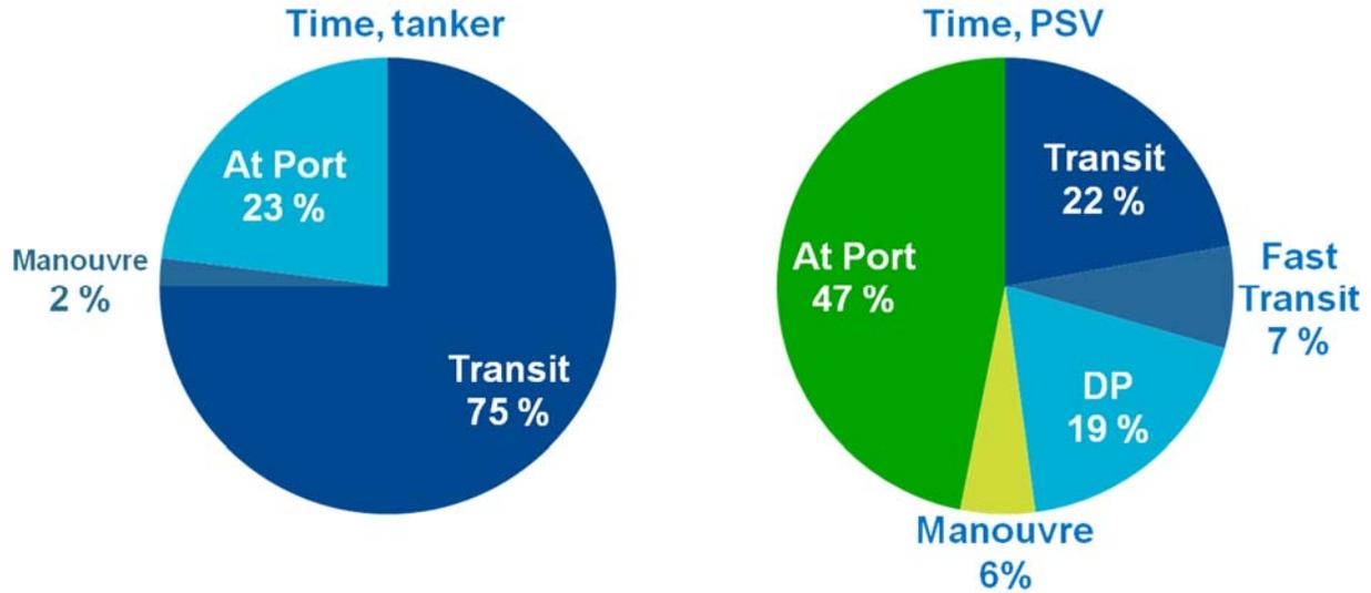
The vessels spend time at sea very differently. The tanker moves on longer legs between ports while the OSV spends a significant amount of time in DP mode and moves shorter distances between several installations and ports.
