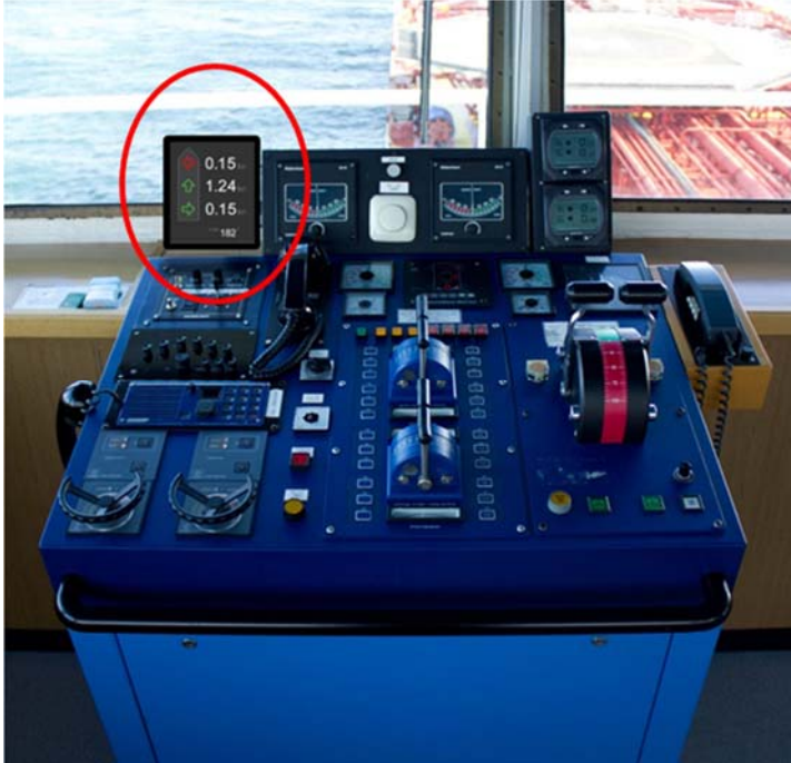
Figure 6: Mock-up display in operational environment
