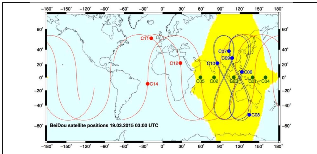
**Fig. 4. Ground track for BeiDou satellites and geographical area with BeiDou 24/7 coverage (PDOP<8)**
