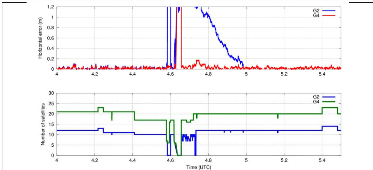
**Fig. 10. Horizontal positioning results for Seoul (South Korea) in presence of RF interference.**
