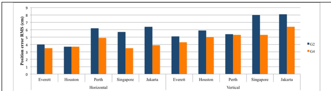
**Fig. 9. Accuracy statistics for different locations, using the legacy G2 solution and the new G4 service**
