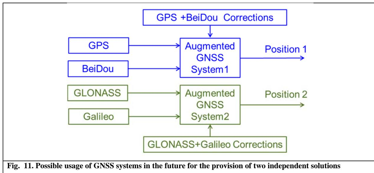
**Fig. 11. Possible usage of GNSS systems in the future for the provision of two independent solutions**
