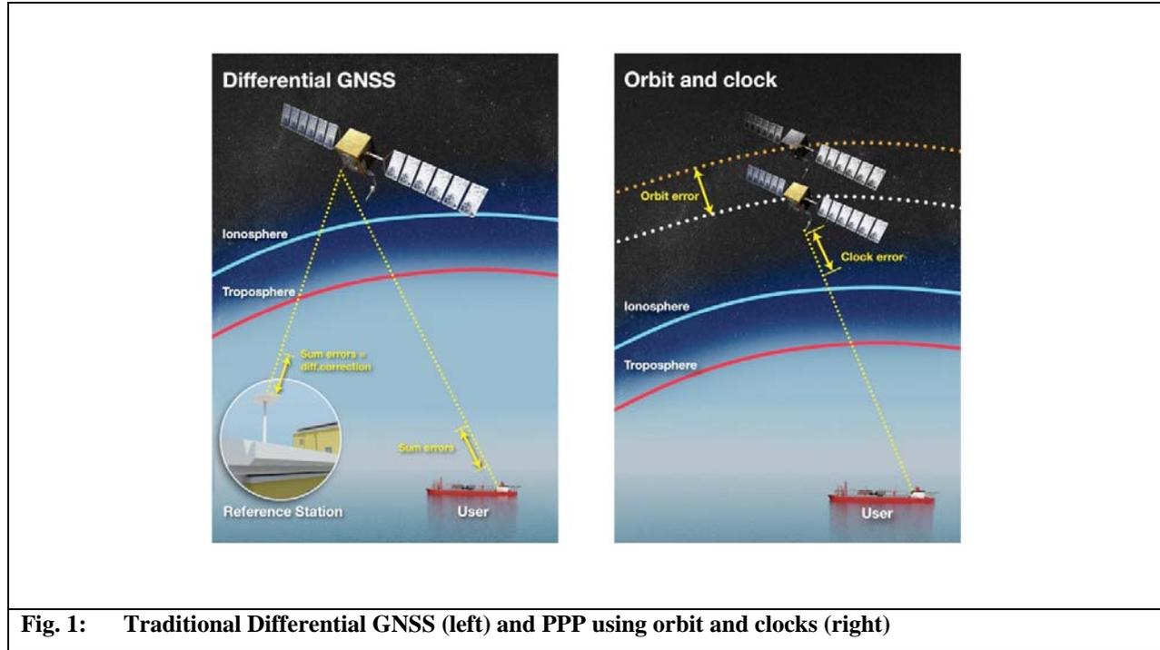
**Fig. 1: Traditional Differential GNSS (left) and PPP using orbit and clocks (right)**
