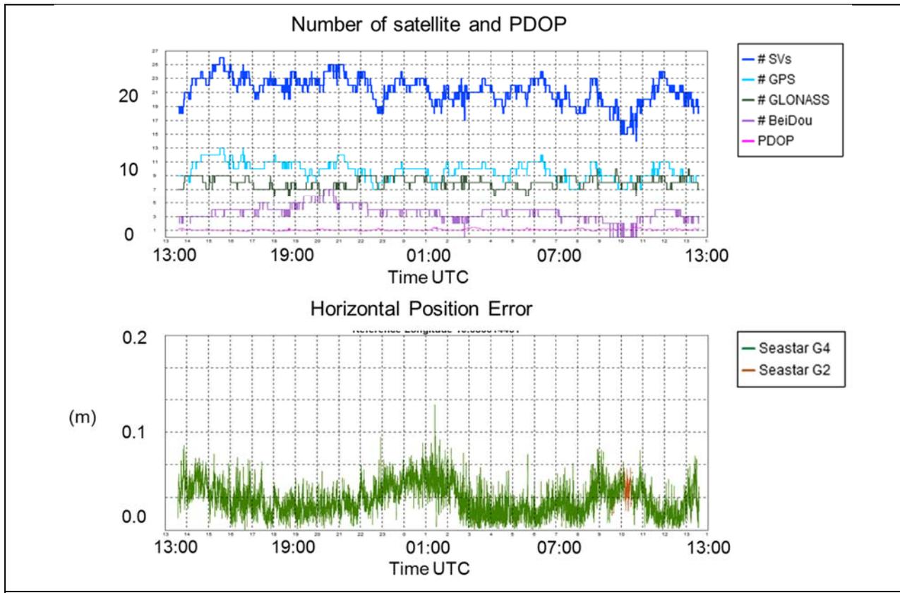
Fig. 8. Example of PPP results using GPS, GLONASS and BeiDou satellites in Oslo (Norway), on July 30-31 2015.
