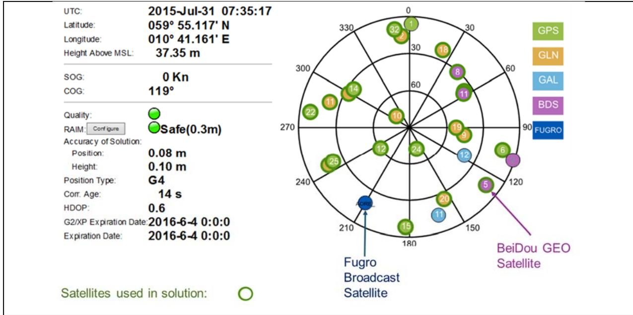
Fig. 7. Example of satellite coverage using GPS, GLONASS and BeiDou satellites in Oslo (Norway), on 31 July 2015.
