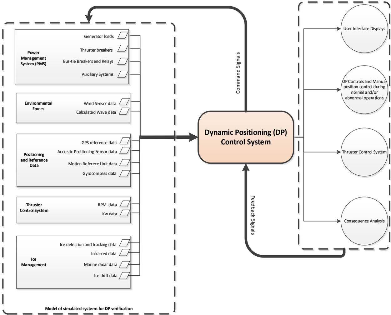
Figure 2: DP Control system model with ice management inputs
