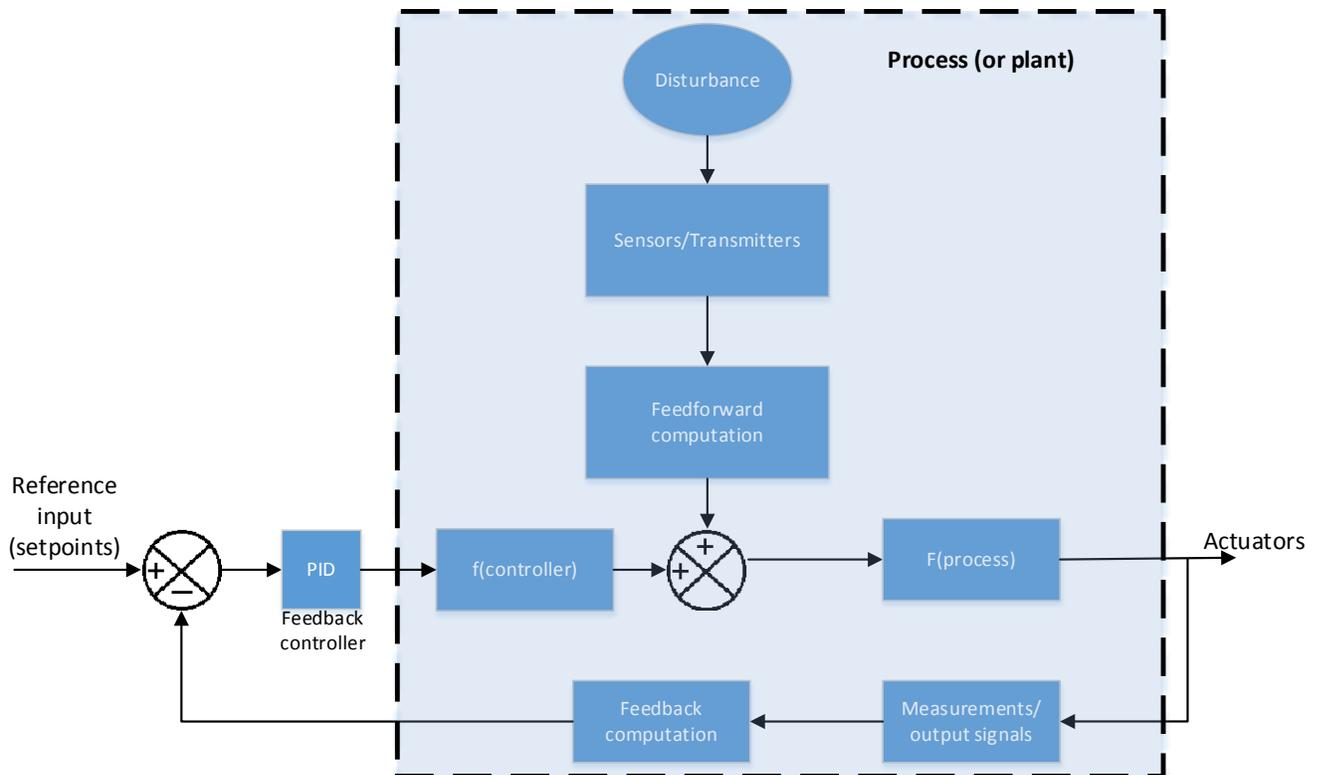
Figure 1: A block diagram of feedback and feedforward control system
