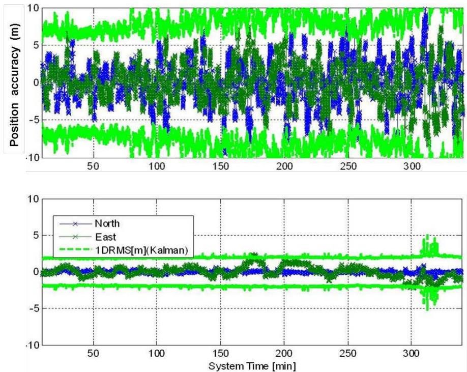
Worse case loosely coupled acoustic inertial accuracy > 5m
