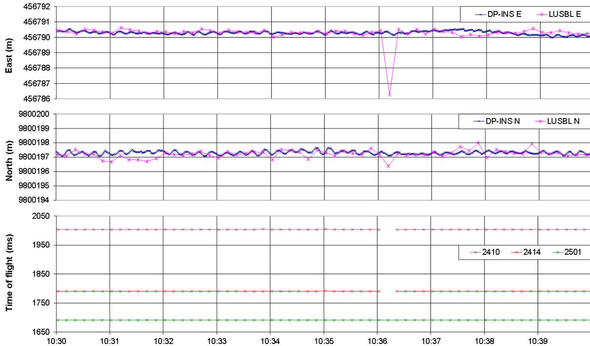
Figure 5 : LUSBL fix degrading to USBL
