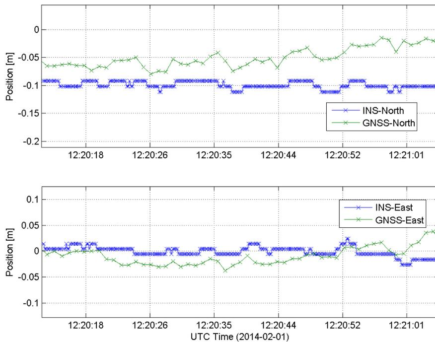
**Figure 11 : INS position stability can cause "freeze alarms" in some DP systems using legacy telegrams**
