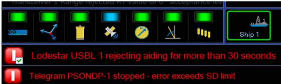
Figure 12 : Alarms reporting loss of aiding and exceeding error thresholds
