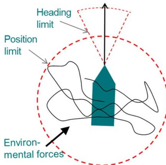
Figure 1: Example of heading and position acceptance limits
