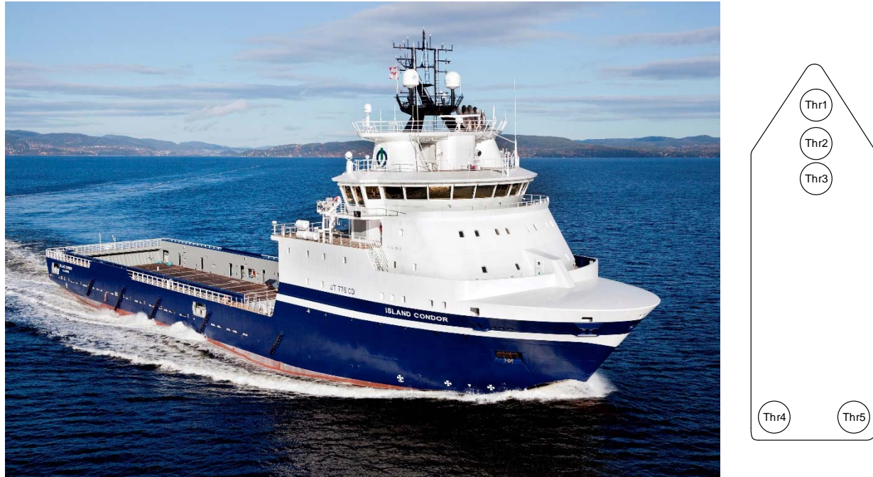
Figure 2: MV Island Condor[14] and thruster layout
