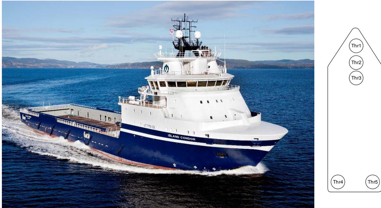
Figure 2: MV Island Condor[14] and thruster layout
