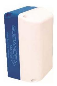
RangeGuard is a 24GHz FMCW radar available from Guidance Marine which is packaged for the marine environment. The range resolution is 0.75m. Range to a point target can be measured much more accurately: down to the nearest inch. It has high sensitivity and low noise, essential for detecting objects challenging to short range microwave radar, such as the bow of a ship.
