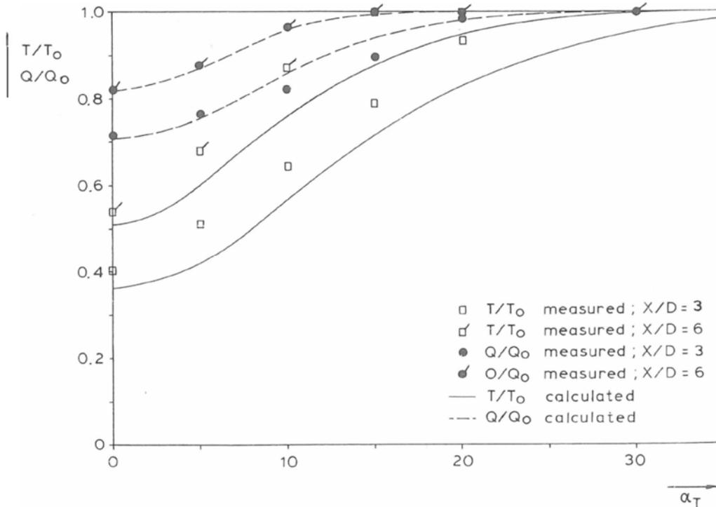
Figure 2 - Interaction as a Function of Azimuth Angle for a Pair of Thrusters - Nienhuis (1992)
