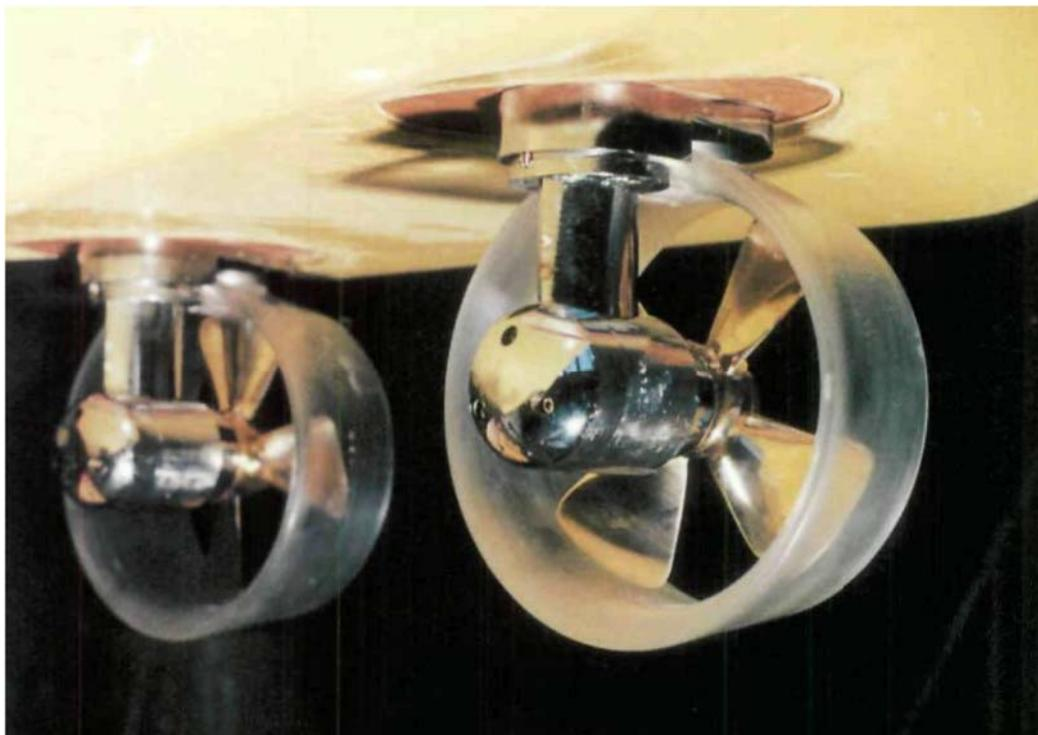
**Figure 1 - First Generation Model Azimuthing Thrusters for DP - MARIN Photo No. F854763 (1985)**
