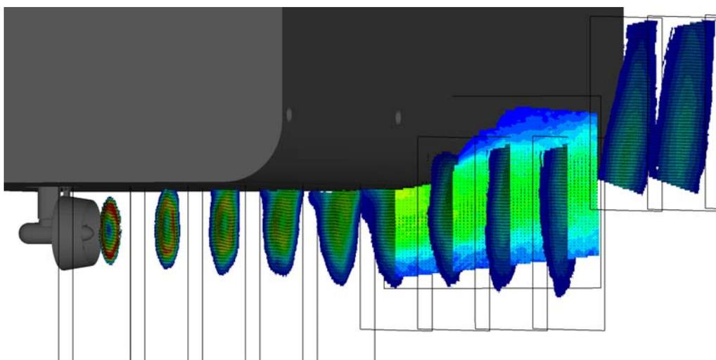
**Figure 4 - PIV Measurements for a Thruster under a Barge - Cozijn and Hallmann (2014)**
