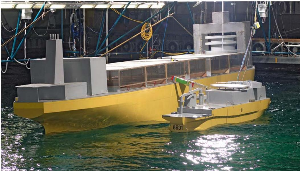
*Figure 6 - DP Accommodation Vessel next to Turret Moored FPSO - MARIN Photo No. 61704 (2006)*
