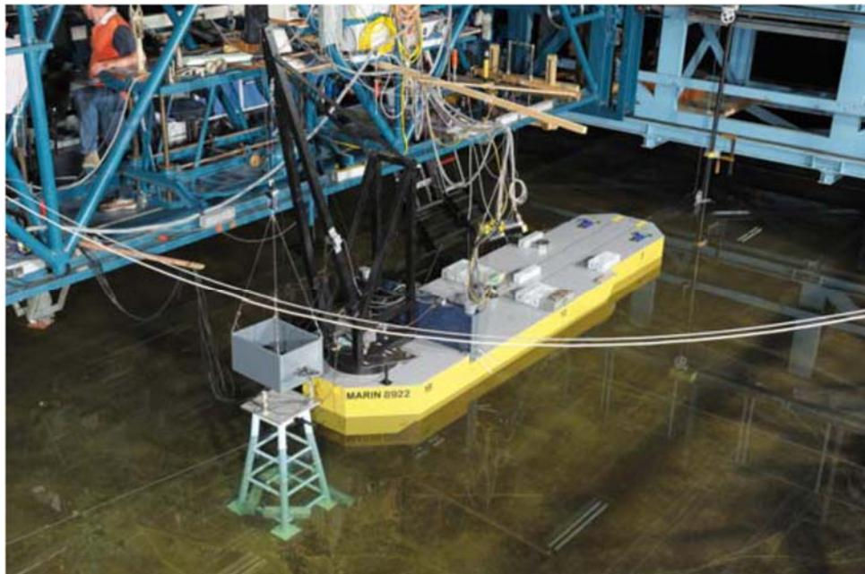
*Figure 5 - Heavy Lift Model Tests with DP Crane Vessel - Waals (2010)*
