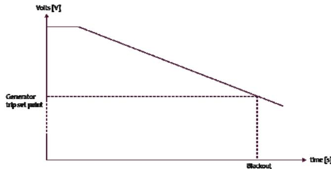
Figure 1 – Blackout Recovery Test – Controlled reduction in a generator terminal voltage
