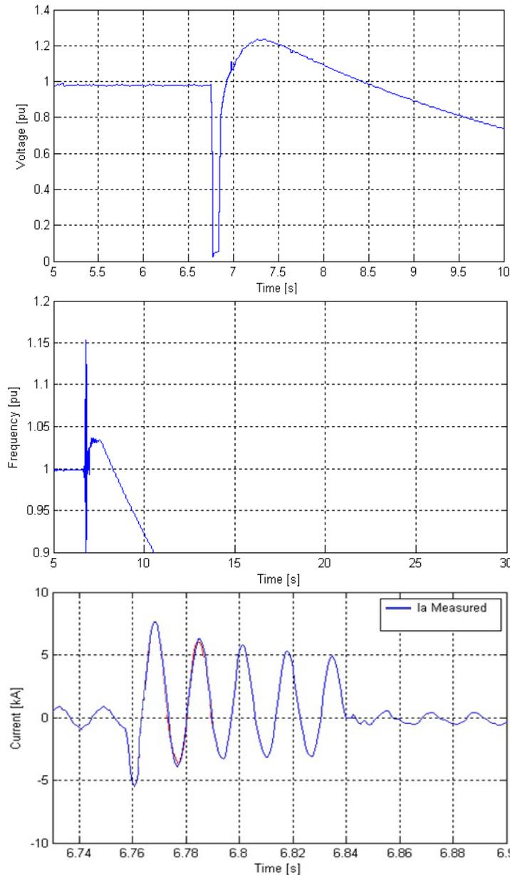
Figure 2 - Voltage, frequency and current disturbances during a fault
