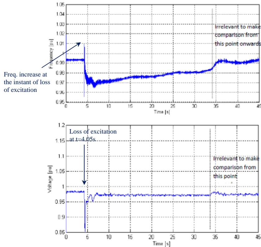
Figure 3 – Voltage and frequency during loss of excitation on one generator whilst operating in parallel
