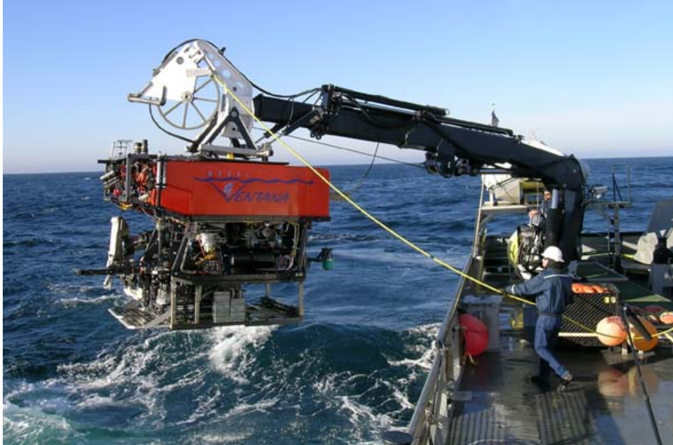
Figure 3: It can be a challenging job to keep the correct positioning of a vessel on Joystick control when the vessel should rotate around a hanging load.
