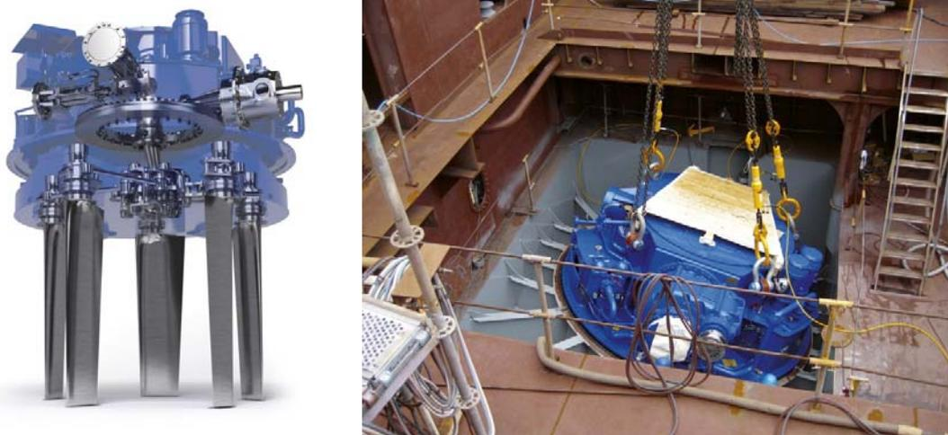
**Fig. 6 Voith Schneider kinematics and installation of VSP into a vessel**
