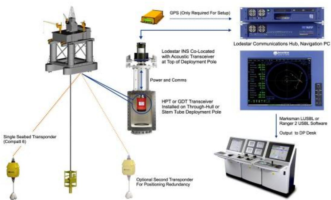
Figure 1: DP-INS USBL system configuration
