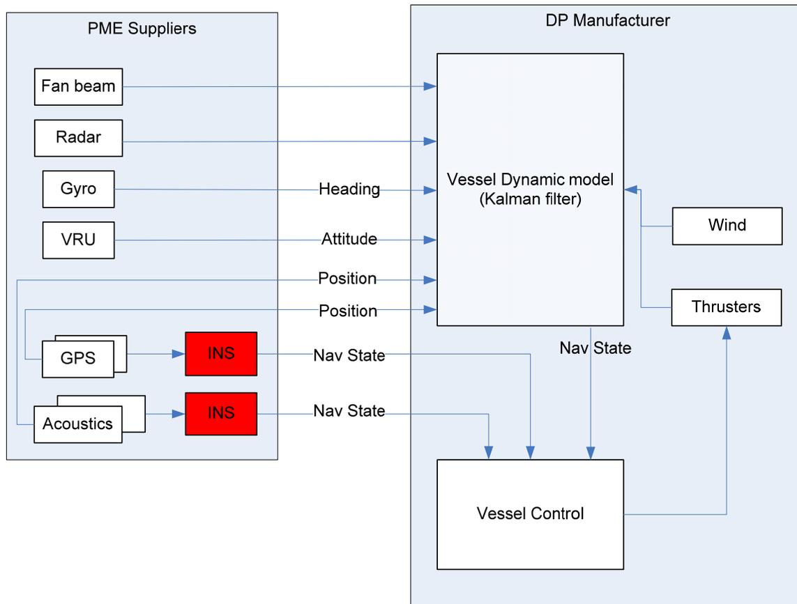
*Figure 11: Candidate architecture for closer integration of INS*
