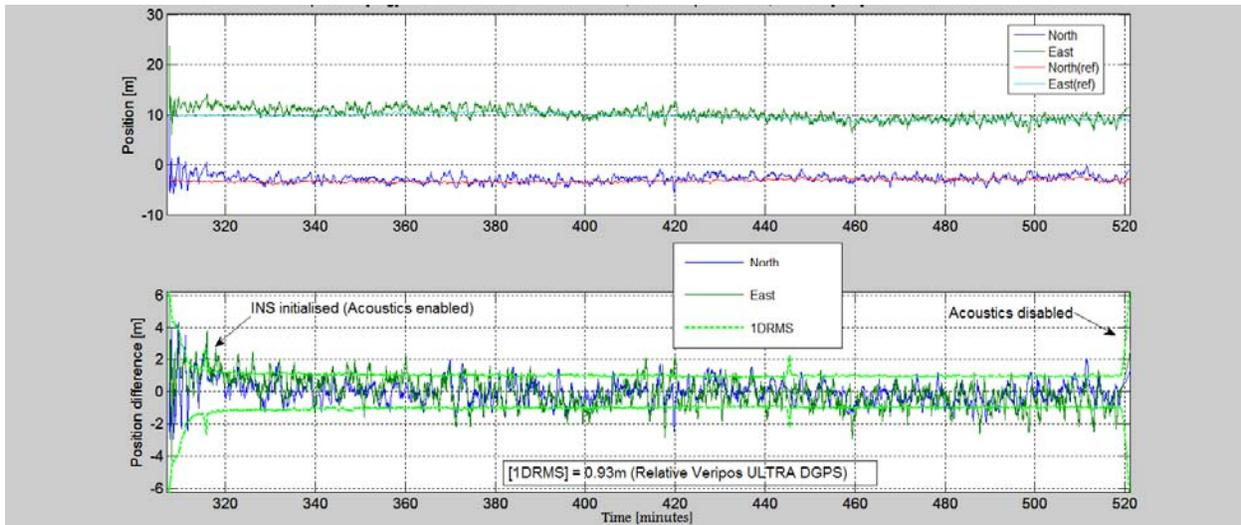
Figure 8: DP INS vs Veripos ULTRA GNSS
