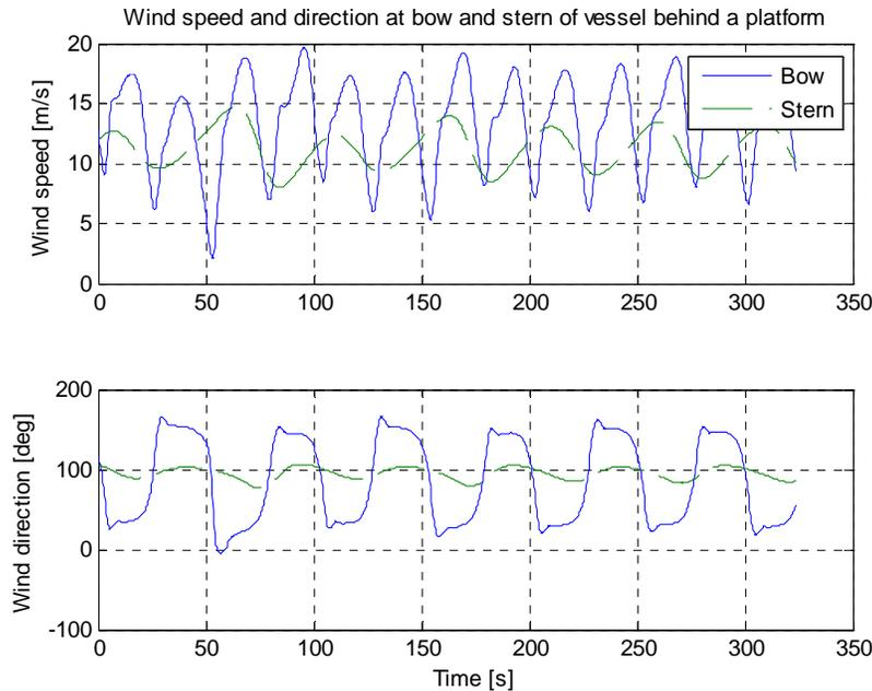
**Figure 4: time variation of wind speed and direction for vessel in lee of platform**
