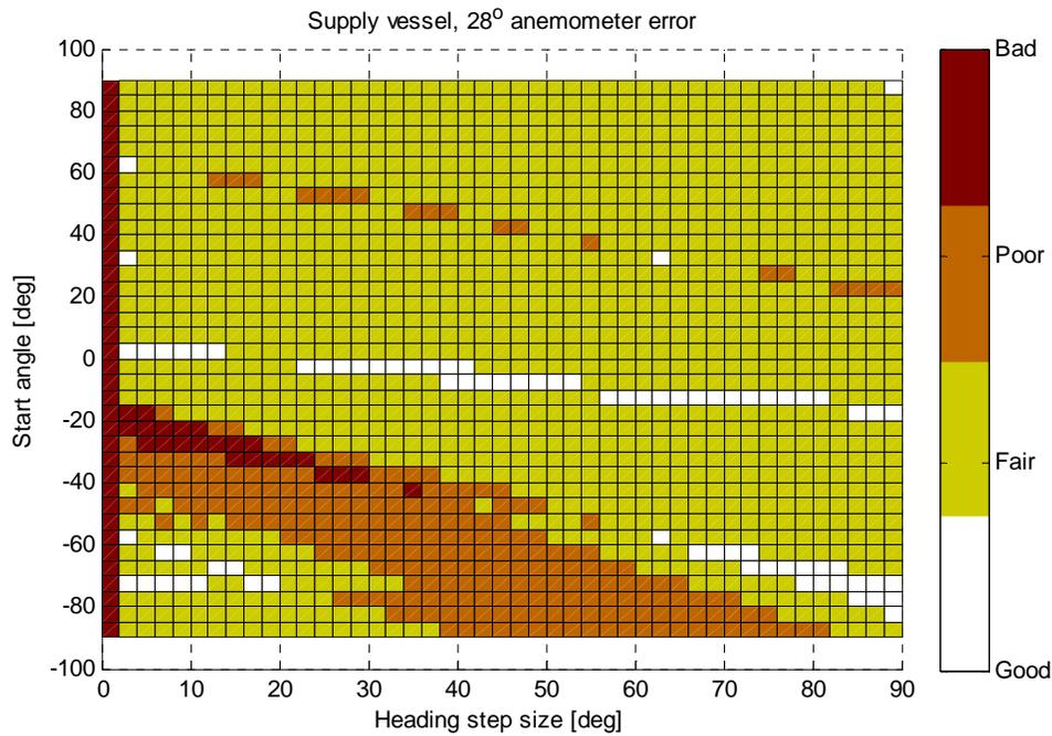
**Figure 6: effectiveness map, supply vessel with 28° anemometer error**
