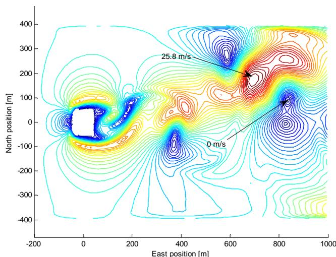
**Figure 3: wind speed variation in the region of a static platform**
