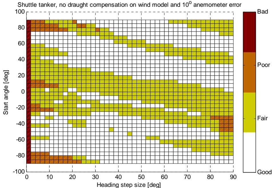
**Figure 9:** shuttle tanker, no draught compensation on wind coefficients,  $10^\circ$  anemometer error
