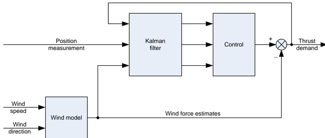
**Figure 1: use of wind feedforward in DP controller**
