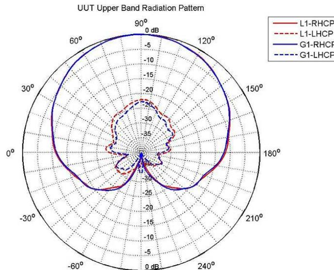
Figure 1 - Gain Pattern for NovAtel 730-GGG Antenna
