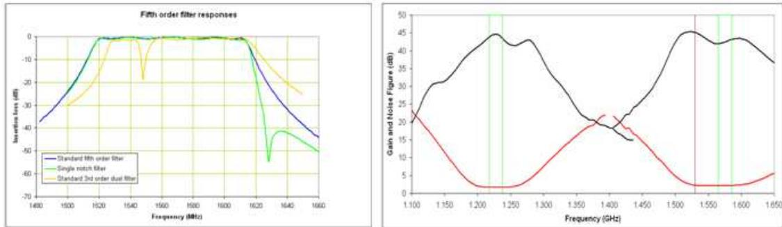
Figure 3 - Filter Response for AD491 (left) and AD410 (right)
