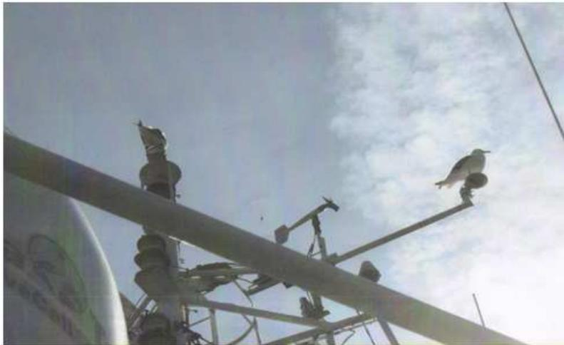
**Figure 9- Interference caused by Birds Sitting on Antenna**
