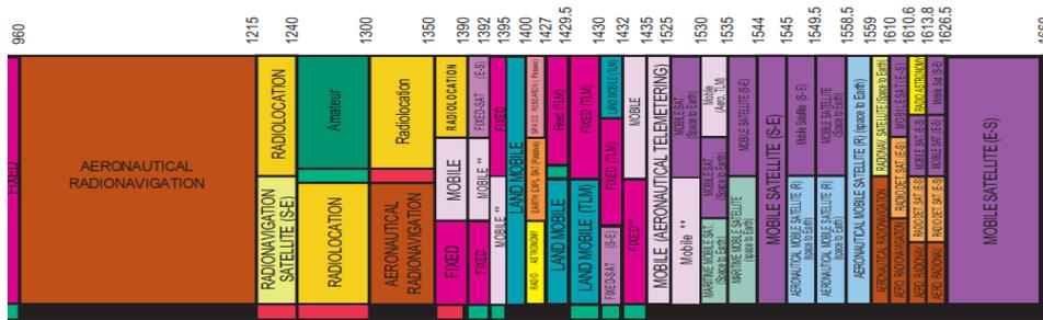
Figure 7 - Radio Spectrum for Satellite Navigation
