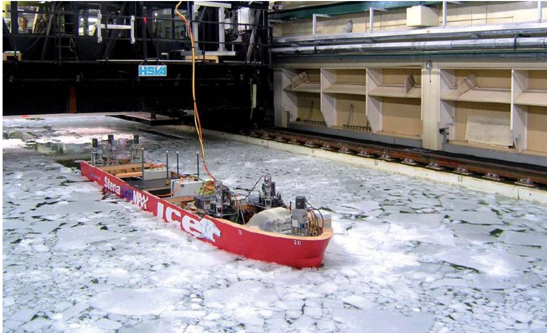
Figure 5: Model of Stena DrillMAX ICE in the model tank at HSVA
