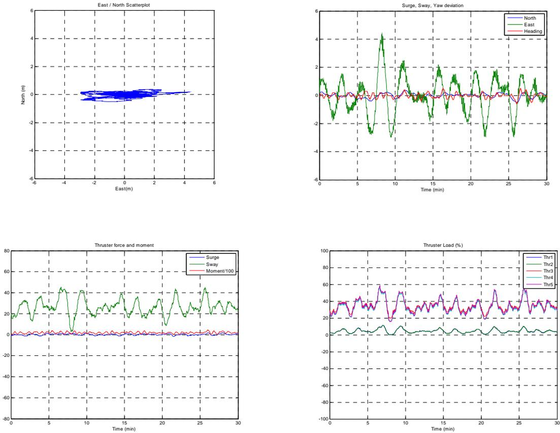
**Figure 4: Scatter Plot for Case 12 listed in Table 5 (top left). Position and Heading Deviation (top right). Thruster Force (tf) and moment (tfm/100), bottom left. Thruster Load (top right)**
