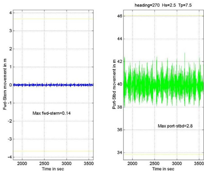
Figure 3: Times series of the gangway movement,  $H_s=2.5\text{m}$ ,  $T_p=7.5\text{ sec}$ , beam sea
