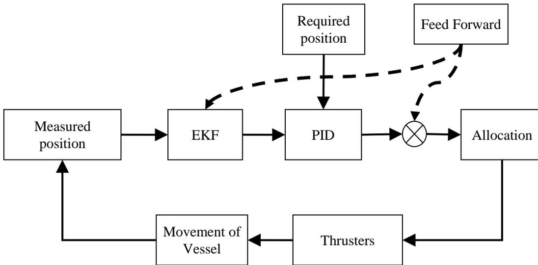
Figure 3: DP control loop with wind feed forward
