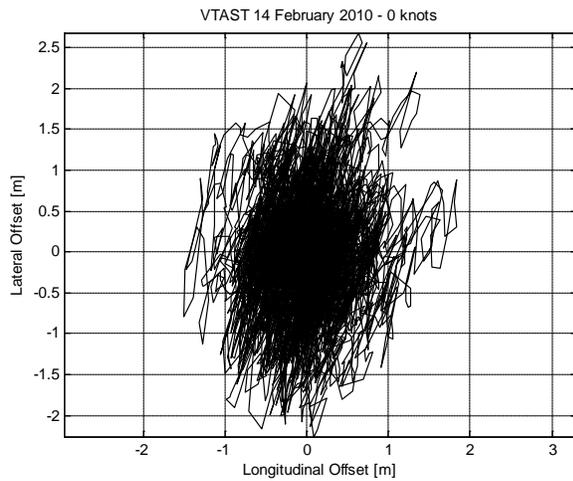
Figure 11: Relative Watch Circle between MS3 and LMSR, 0 Knots
