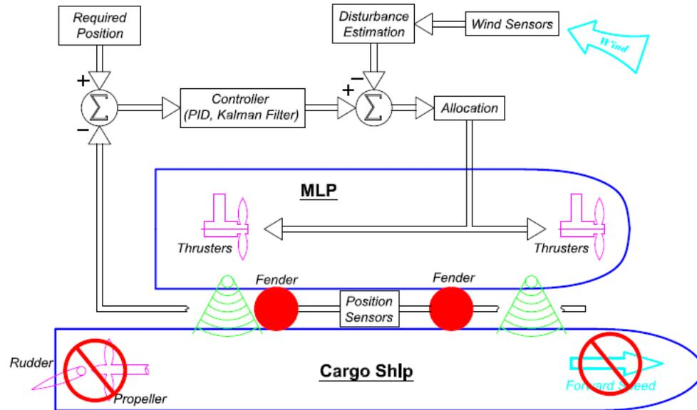
Figure 14: DP controller arrangement for DP Pushing
