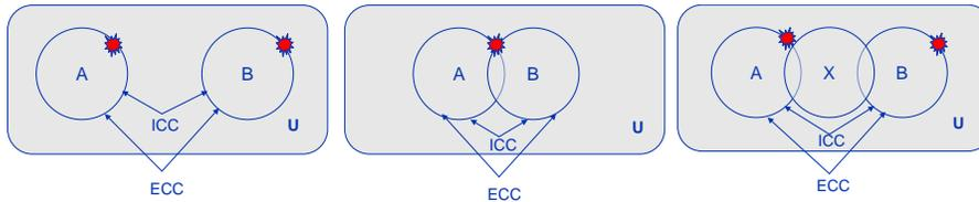
Fig.7. Common cause failure, resulting from a single event related to U, e.g. either as an external (ECC) or an (ICC) internal common cause. (E.g. fire and flooding, environment, vibration, high seas affecting contamination in fuel tanks, shocks, humidity, EMC,....)
