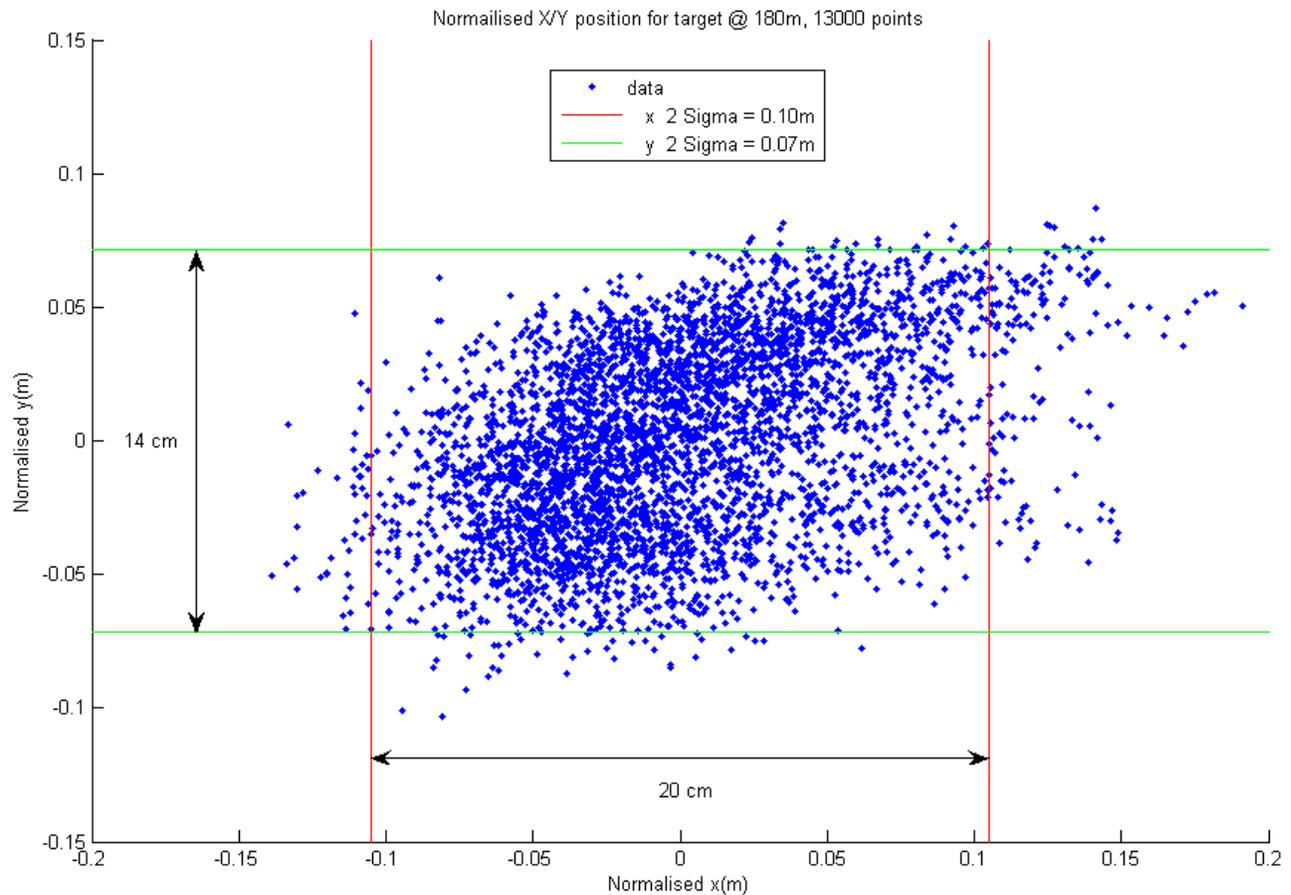
**Figure 4: RadaScan transponder position plot at 180m (590feet)**
