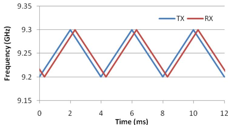
**Figure 2: RadaScan FMCW Radar Output and Return Signals**
