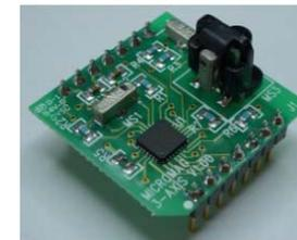
PRO-Series Controller (L-3 DP&CS) 3-Axis Magnetometer (MicroMag)
