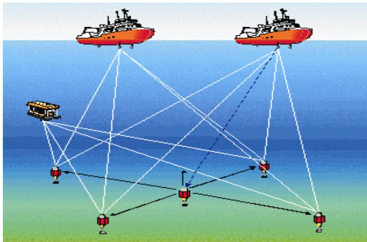
Typical Multi User configuration ( one array with master transponder in the middle ).
