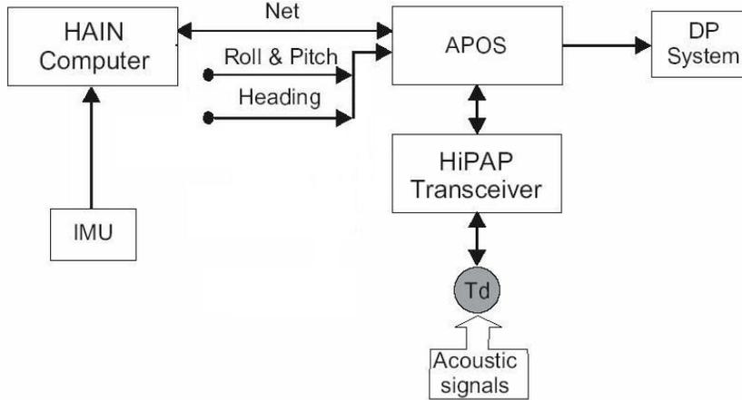
Configuration of a Hydroacoustic aided inertial system, one extra computer is needed to calculate the aided positions.
