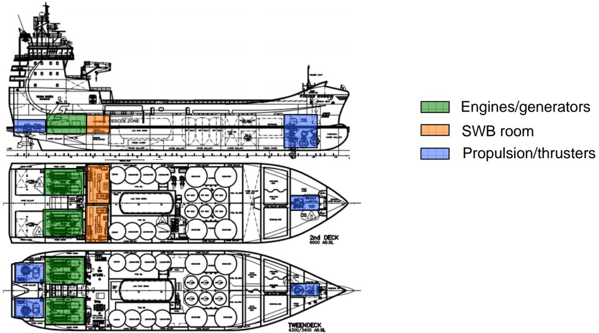
Fig 4. Viking Queen – Machinery and Propulsion arrangement
