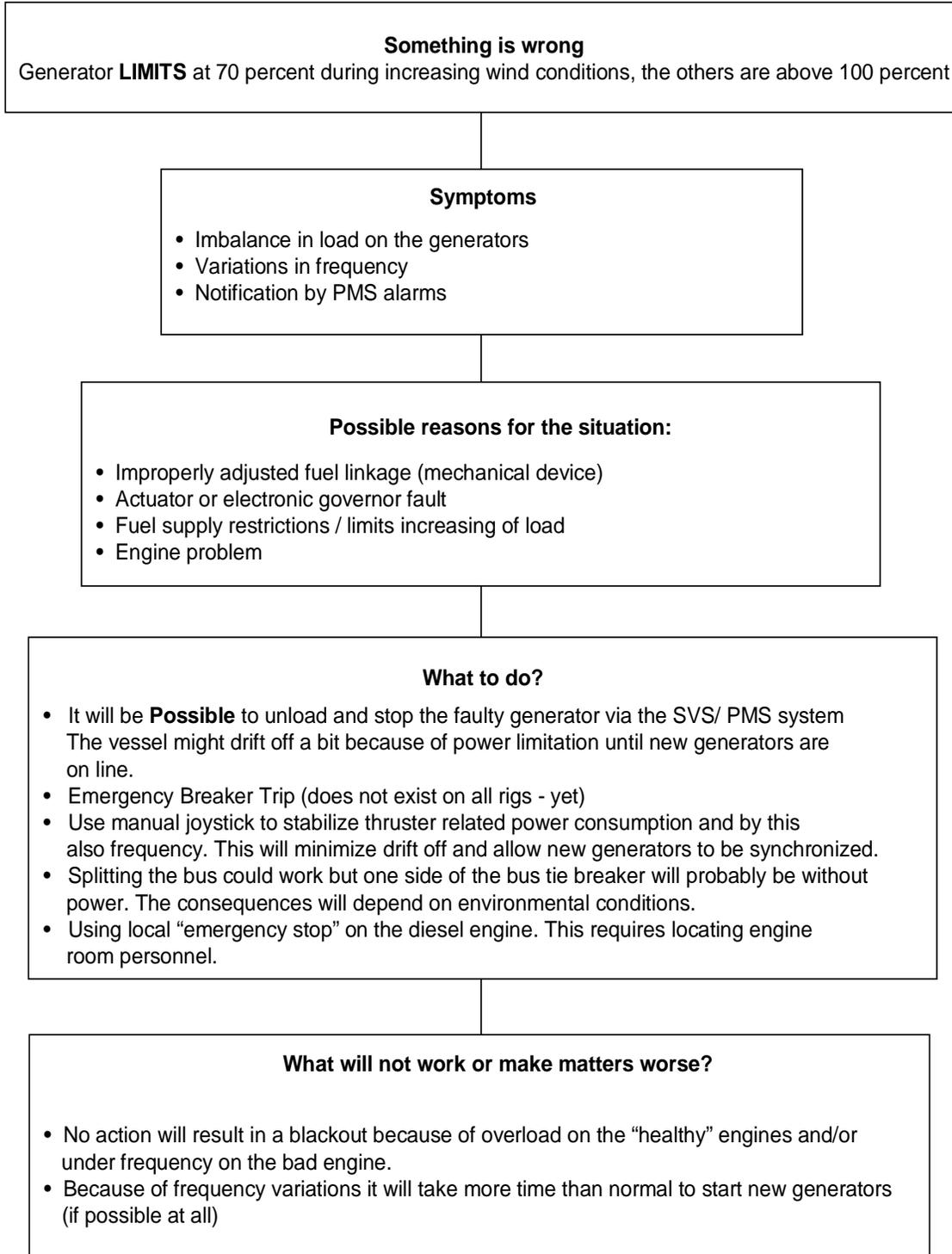
**Figure 4.** Example of a similar scenario and the different actions to take to illustrate the importance of understanding vessel automation versus memorization of actions to take.
