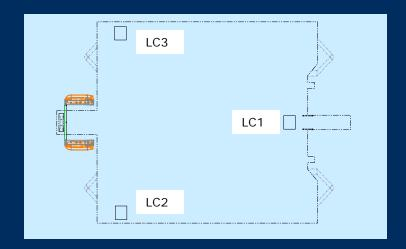
Three sets of dual-axis load cells were used to measure thrust forces during thruster-hull and thruster-thruster interaction tests.
