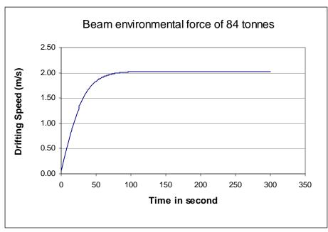
Again assuming the vessel operates between 10 to 30 m from the platforms, taking three points off the curve gave the following impact velocities.
