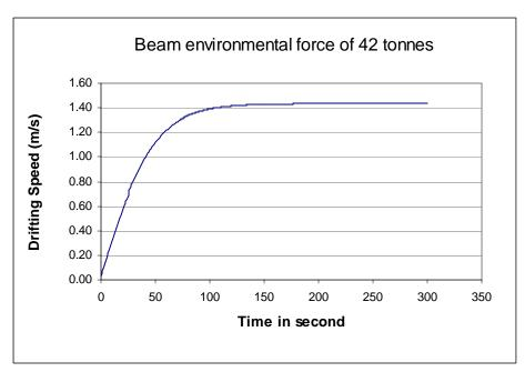
The vessel will be operating at up to 30 m from the platforms and as close as 10m, taking three points off the curve the impact velocities are
