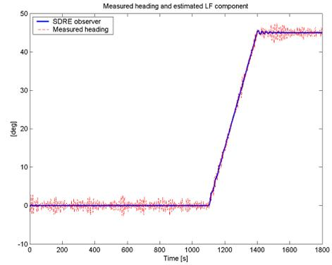
Figure 8: LF estimation using the SDRE observer and measured heading
