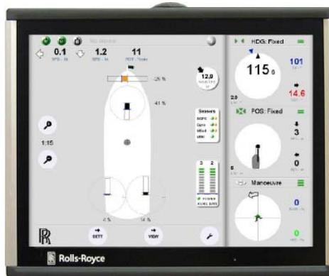
Figure 4. New range of graphical displays, here with a Poscon DP user interface.
