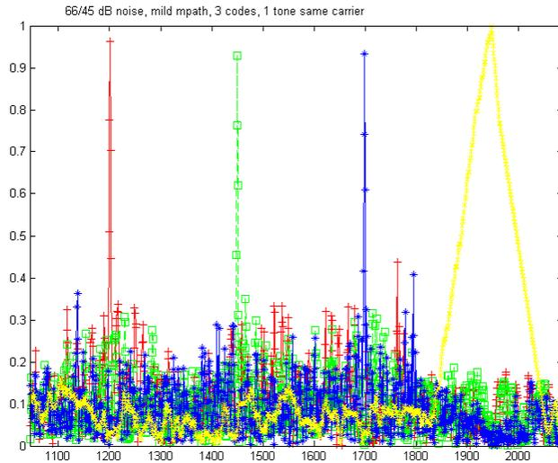
As can be seen from the filter output shown above, the measurement point for the wideband signals (red, green and blue) is a clearly defined point and far easier to process than the tone shown in yellow.
