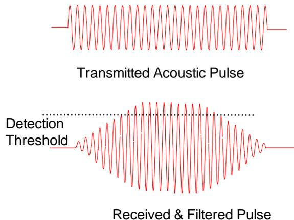
An analogue signal is received when the signal level exceeds a detection threshold in the receiver. As the incoming pulse exceeds this detection threshold, it is then validated and the measurement point is determined. This is shown in the diagram above.
