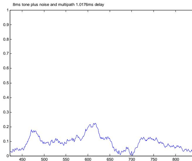
The diagram above illustrates the case where multi-path interference of a narrowband signal has resulted in signal destruction. In this case the signal would not have been detected. In the diagram below signals from two paths have combined (constructive interference). The filter output is flat topped and the time of arrival is ill-defined. It is very difficult to resolve the direction of arrival of both paths.
