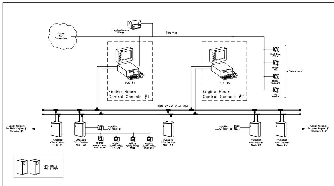
Figure 1 – Typical Workboat VMS System (Nautronix VMS5500)
