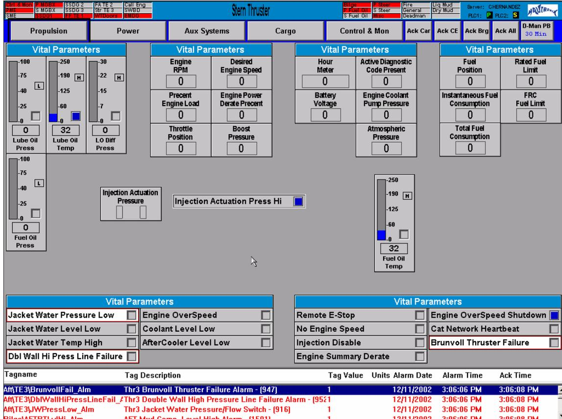
Figure 2 – Thruster Overview Page (Nautronix VMS5500)
