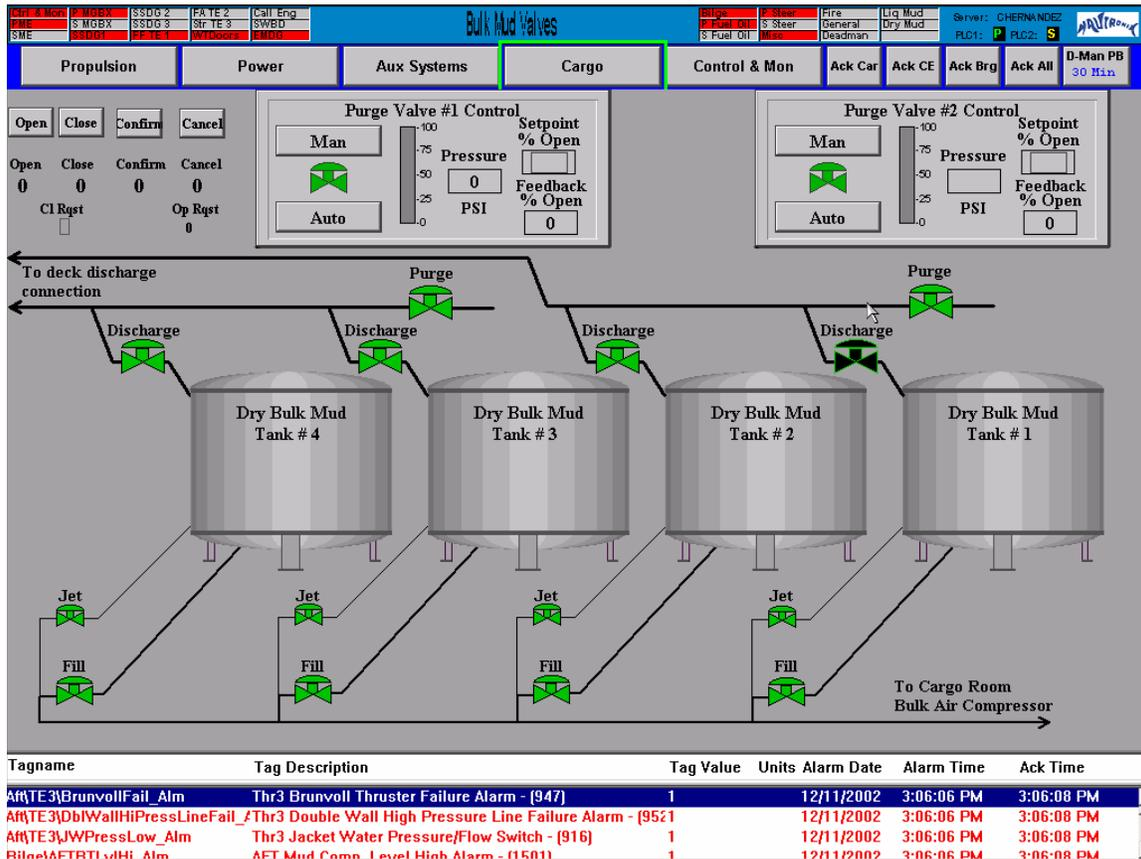
Figure 3 – Bulk Mud Page (Nautronix VMS5500)
