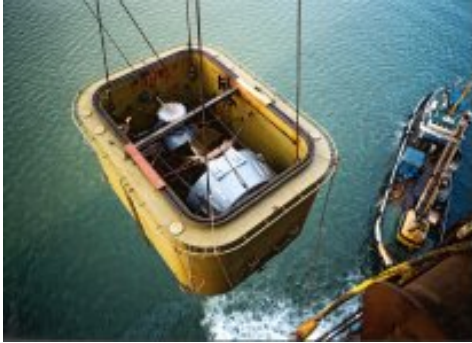
Fig. 2 The installation of the habitat which contains the thruster gearbox, propeller and nozzle.
