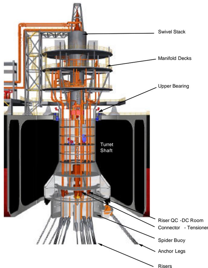
**Figure 3. The Terra Nova disconnectable turret mooring system**
