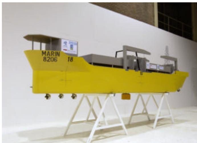
**Figure 5. DP FPSO model with disconnectable buoy**
