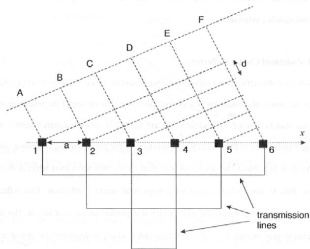
Figure 2: Van-Atta Schematic
