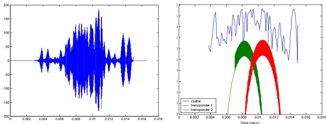
Figure 9: Time domain waveform and power spectrum analysis of two narrowly spaced targets against a background of radar clutter.
