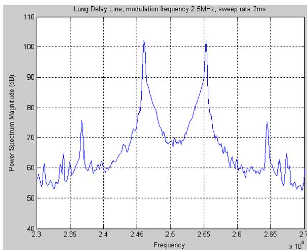
Figure 7: Target at 130m range ( $\Delta \pm 40$  kHz)
