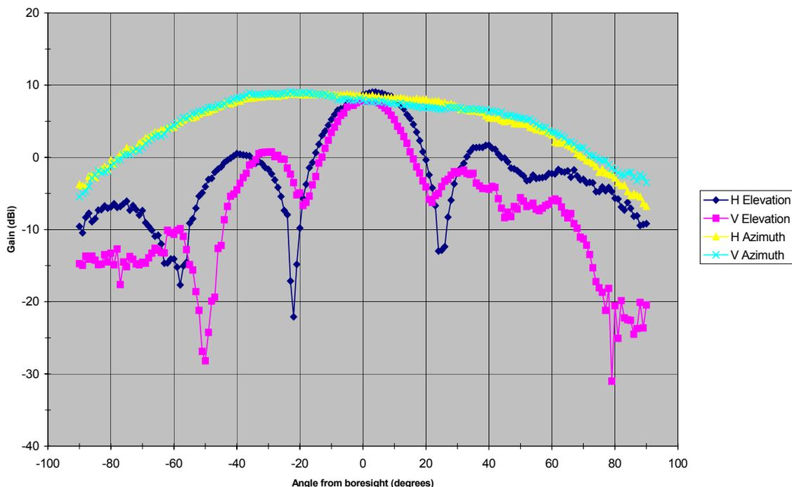
Figure 4: Gain with bore-sight for each polarization
