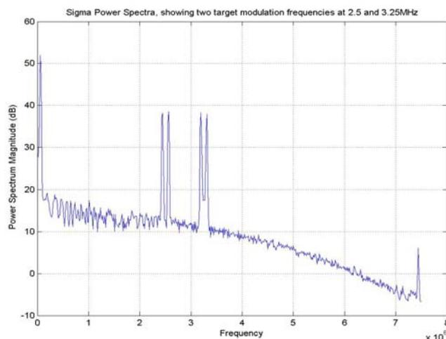
Figure 6: Two target power spectrum
