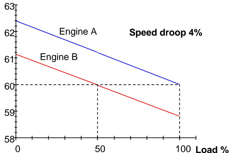
**Engines which are connected to a common load must have the same speed reference and the same speed droop % in order to share the load equally.**
