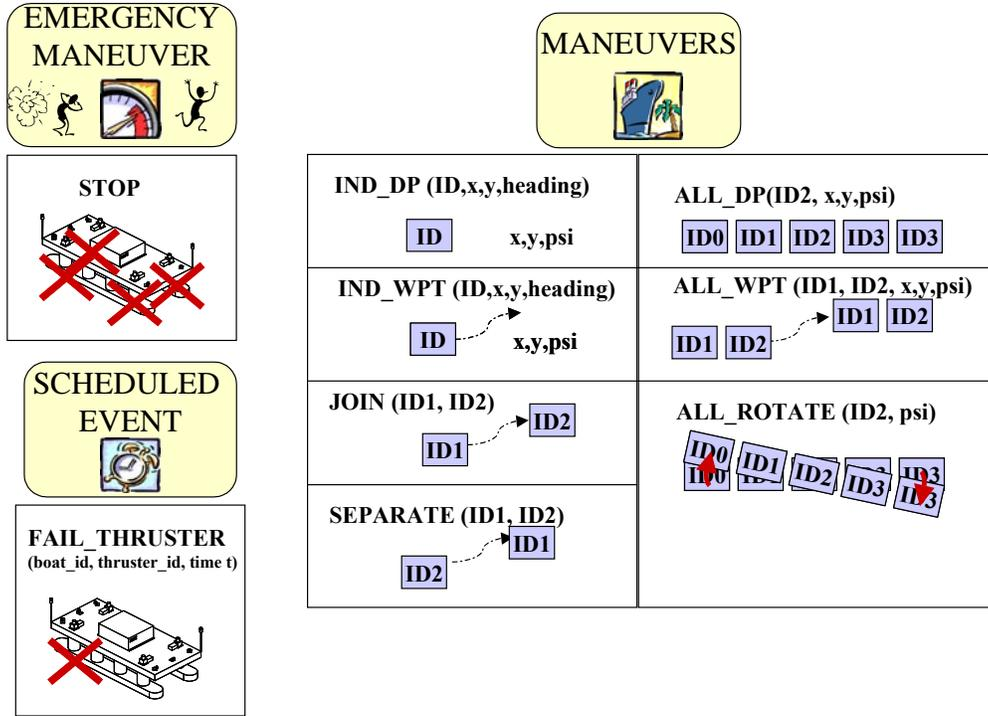
Figure 17. Maneuvers accommodated by the Scaled MOB Testbed.
