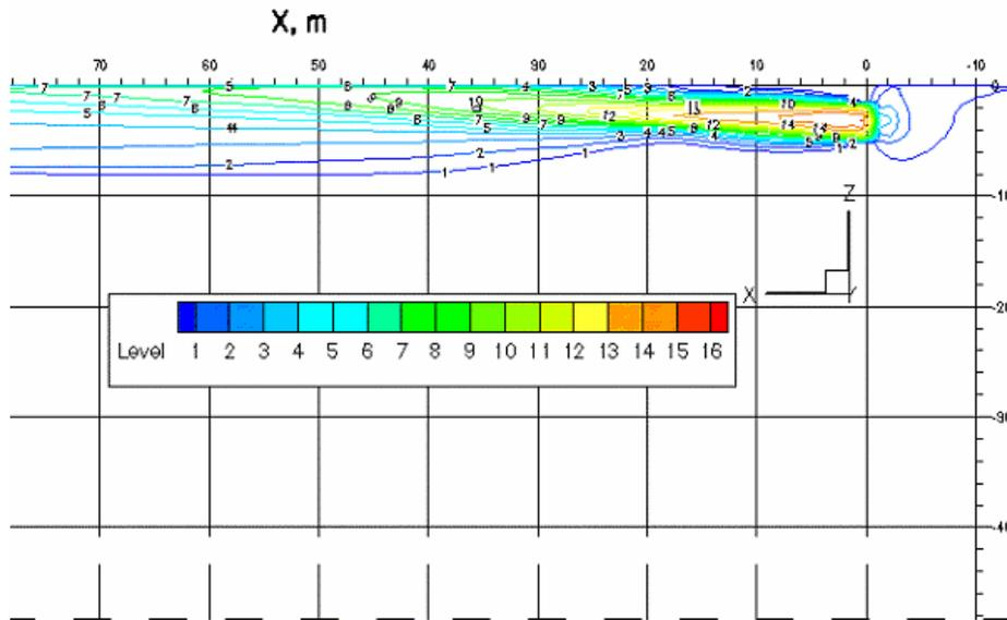
Fig. 10: Distribution of axial velocity  $V_x$  from propeller jet near flat plane.
