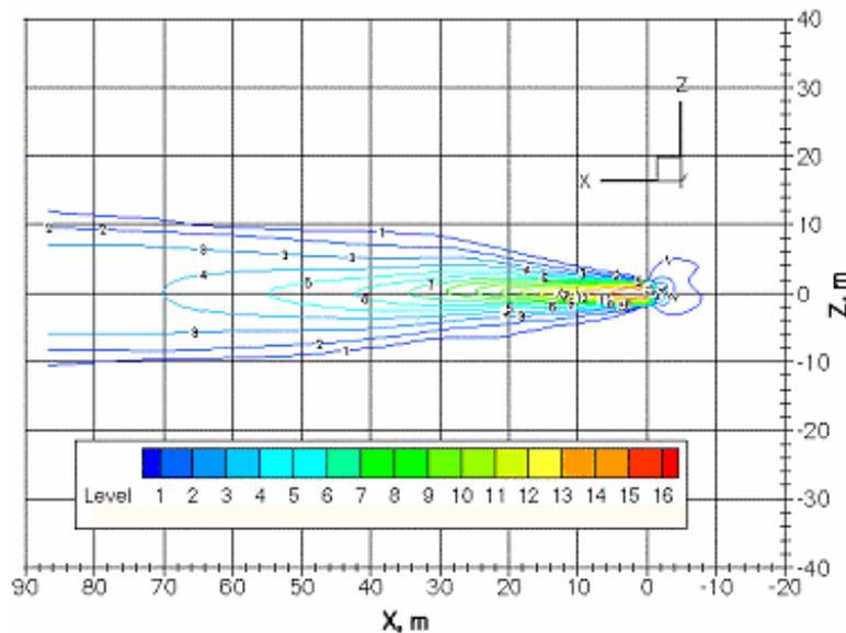
Fig. 8: Distribution of axial velocity  $V_x$  in propeller jet. Model condition.
