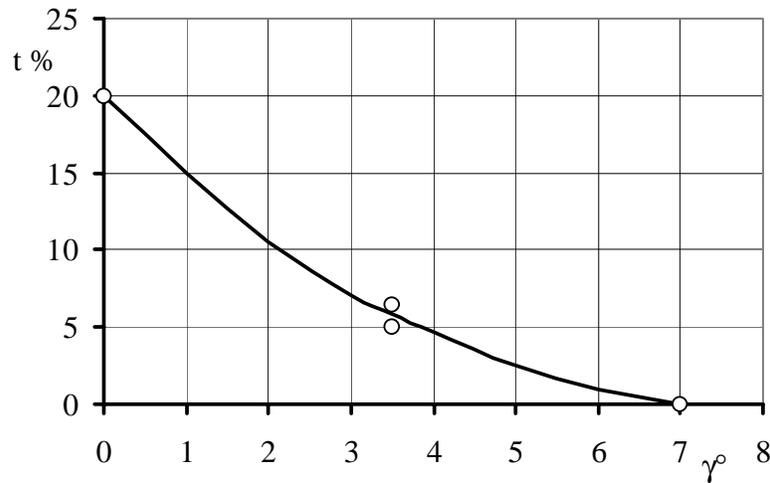
Fig. 14: Thrust deduction coefficient as a function of tilt angle at  $\alpha=0^\circ$
