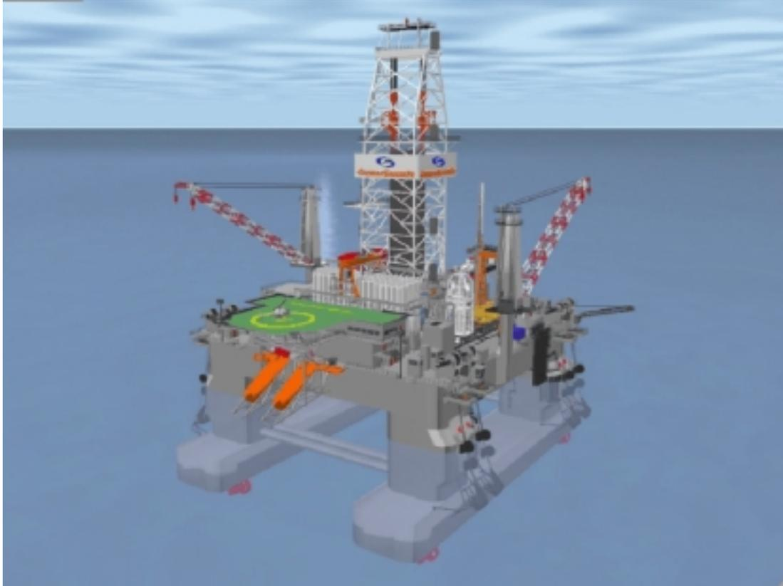
Fig. 1: Development Driller Class semi-submersible.
