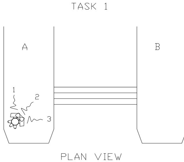
Fig 7. Definition of thruster position and direction of jet/wake relative to pontoons A and B.
