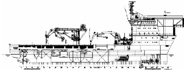
*Fig. 5: GA drawing of the UT 745E multifunctional platform supply and ROV vessel.*
