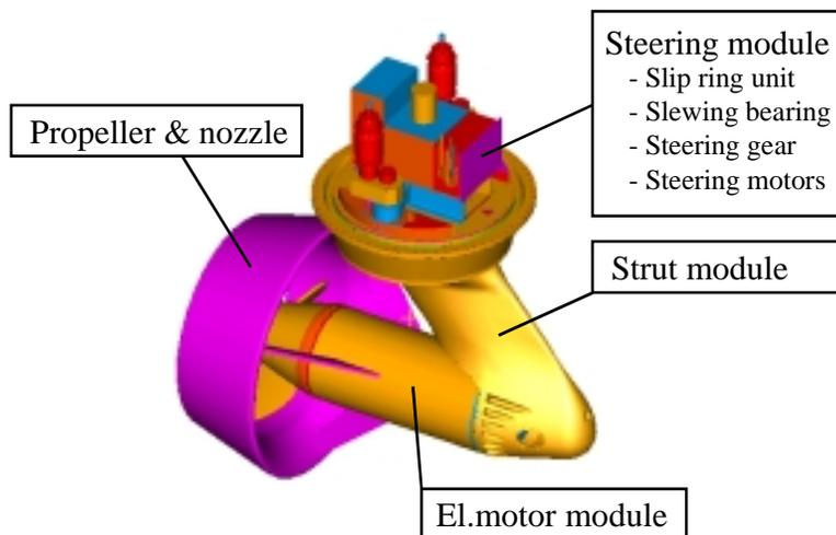
Fig. 4: Compact Azipod thruster.
