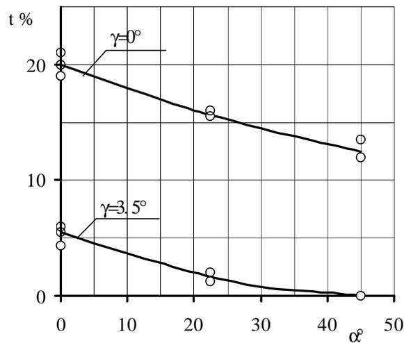
Fig. 15: Thrust deduction coefficient as a function of turning angle.
