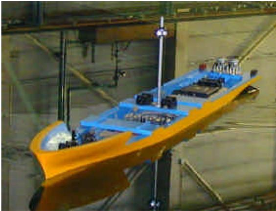
Fig.1 Controlled object (model ship)
