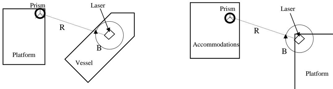
Whether the laser is located on the vessel or on the platform, the laser system operates in the same manner. In dynamic positioning, the laser is located on the vessel in most instances but it can be located on board platforms to track other closely situated structures such as accommodation modules.
