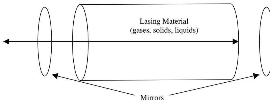
Light from incoherent sources (such as a light bulb) are composed of many different wavelengths traveling in all directions causing the light to spread as it travels so it cannot be focused with precision. Light waves from a laser are in phase with each other. This enables the light from the laser to travel for long distances with little diffusion. This unique coherence property allows the light to be concentrated so it can be focused with greater accuracy.
